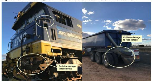
Figure 2: Collision damage to the locomotive and the last trailer of the road-train
