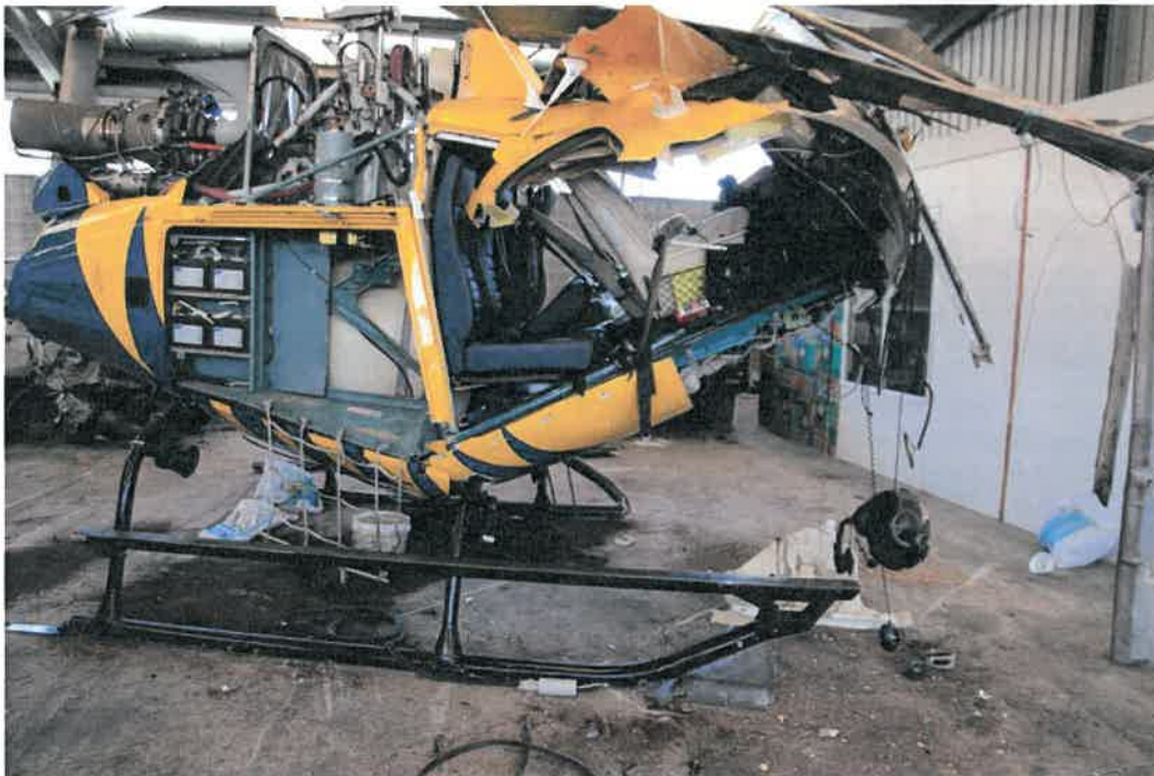
Figure 2: Damage to the helicopter showing significant impact damage to the cockpit area and left landing skid tip, consistent with a left nose-down attitude on impact.
