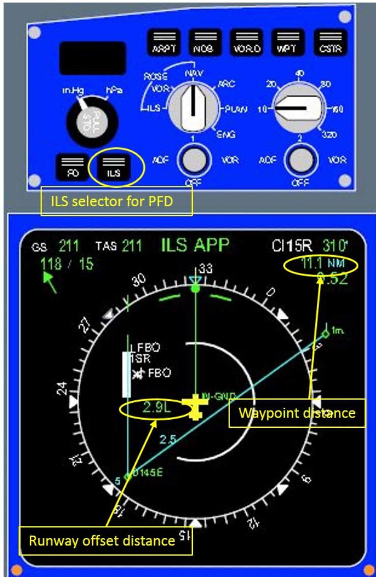
Figure 3: Example of a navigation display (ND) with distance information and cross track error displayed
