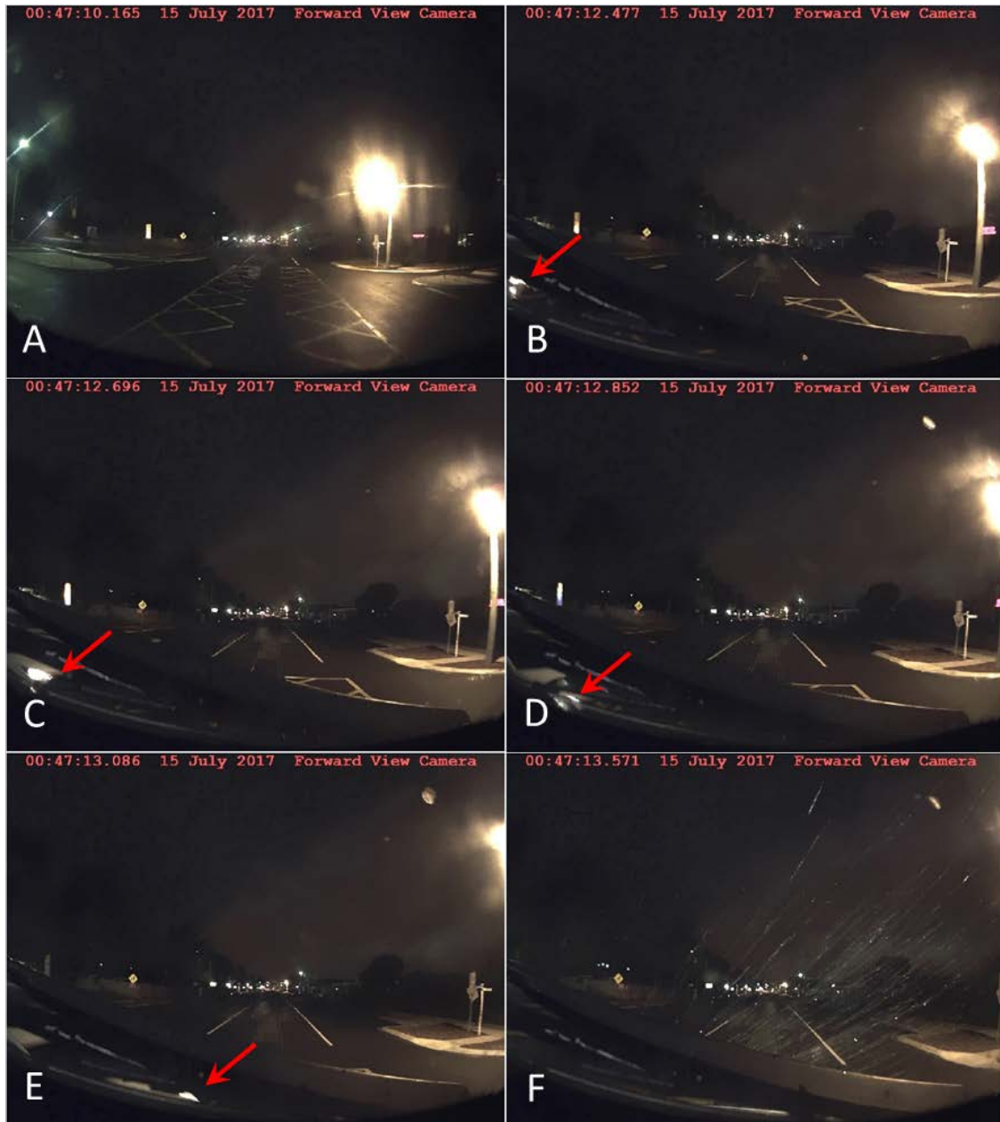
Figure 2: Forward-facing train video camera sequential frames (red arrow shows the position of the road vehicle)
