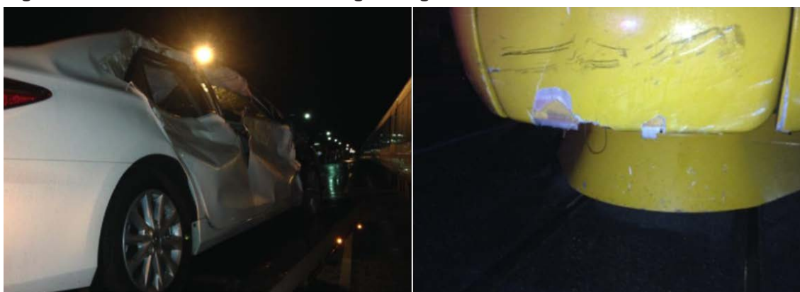
Figure 1: Vehicle and train front cowling damage
