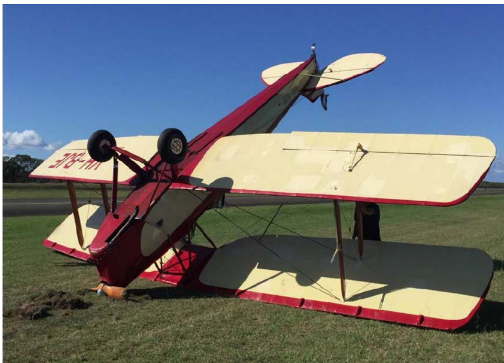
Collision with terrain of a de Havilland DH-82A. Source: Ron Ennis — modified by the ATSB
