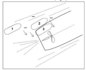
Image shows the simplified distribution of pressure zones around a ship underway (Left) and the effect of interaction on a tug aft (Right) Source: Reproduced with permission from The Shiphandler's Guide, published by the Nautical Institute, modified by the ATSB
