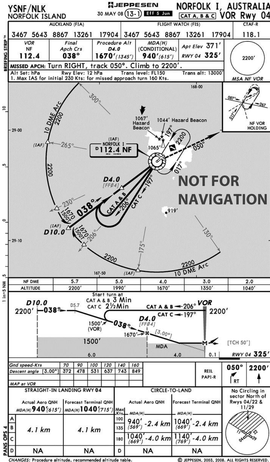
Figure 27: VOR instrument approach procedure to runway 04
