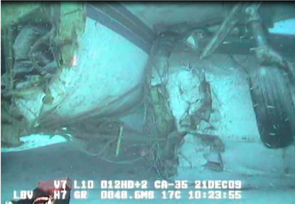
Figure 17: Fuselage separation location and damage to the forward lower fuselage section
