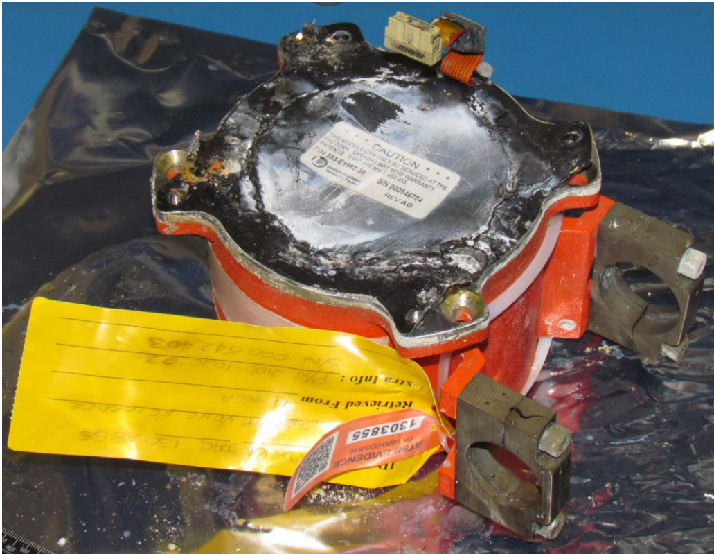
Figure A3: CVR crash-survivable memory unit, 16 November 2015
