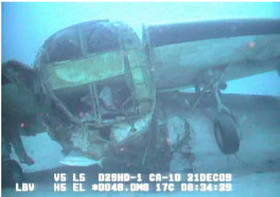
Figure 16: Front-on view of forward fuselage separation point, showing wing spar carry-through structure, main fuselage fuel tanks and damage to the underfloor fuselage section
