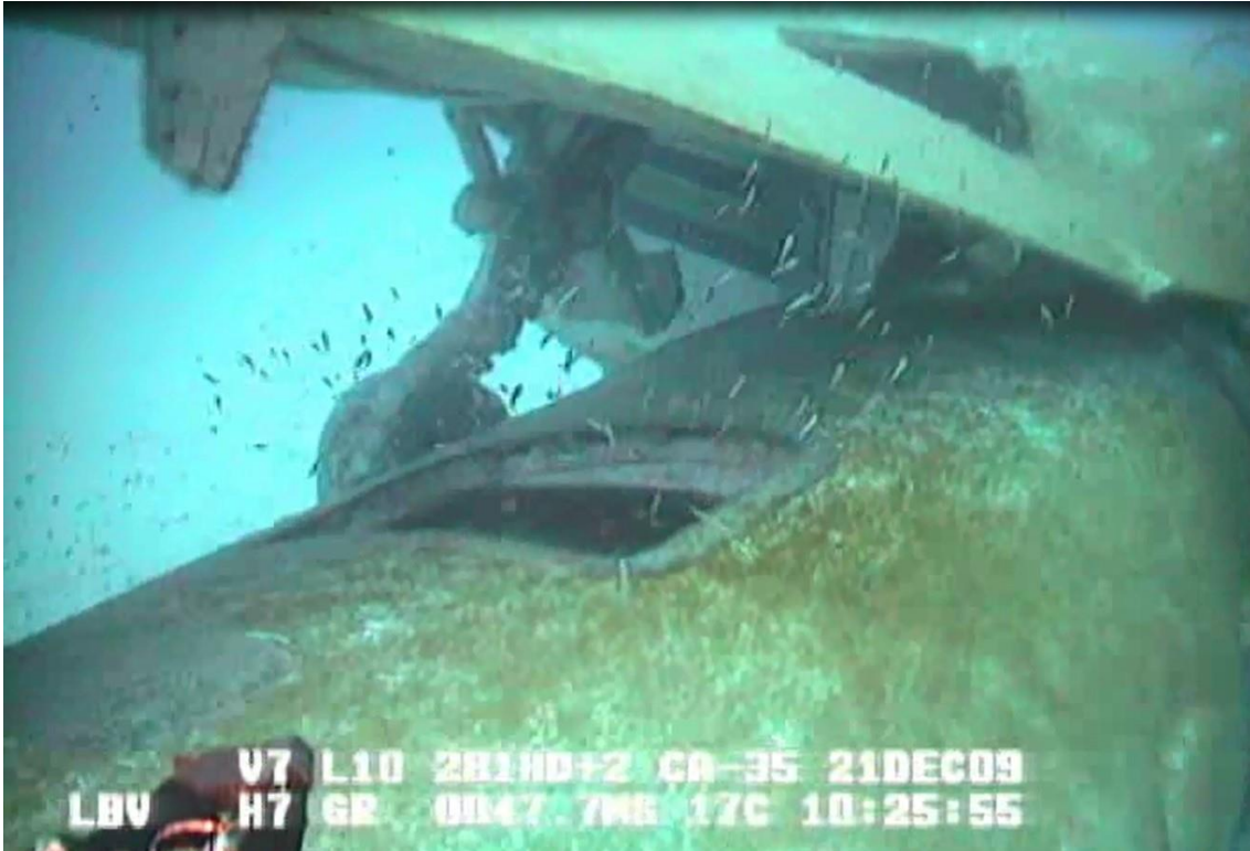
Figure 19: Right side of forward fuselage, showing open emergency exit.
