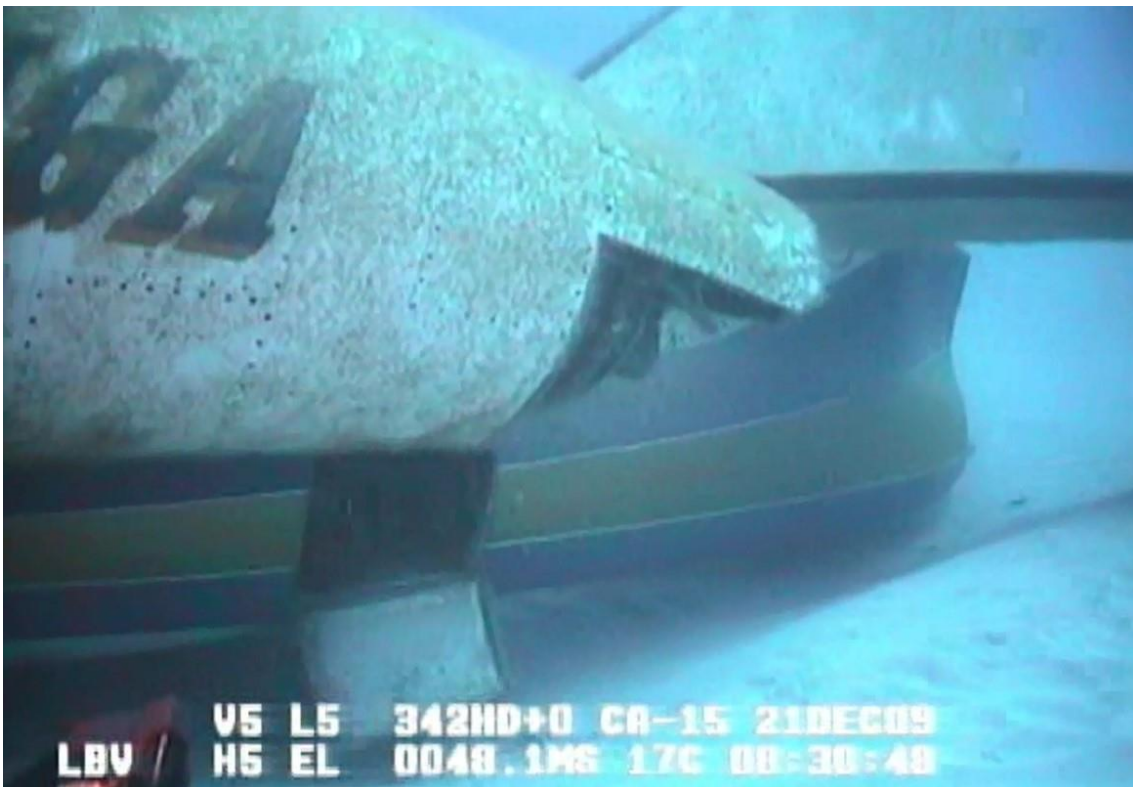
Figure 22: View from left side of rear fuselage, showing open rear baggage compartment door
