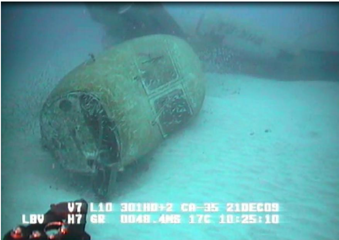
Figure 20: Forward fuselage resting on the seabed on its left side
