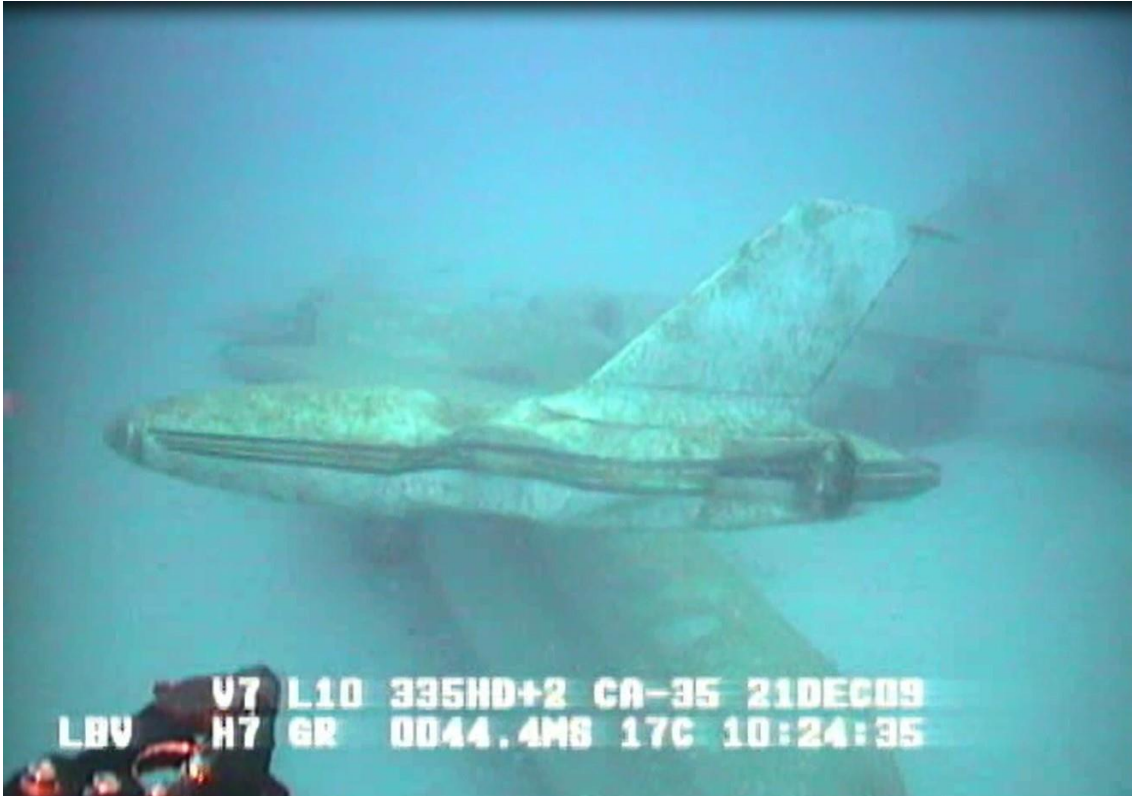
Figure 23: View of left tip tank, showing crushing damage due to water pressure
