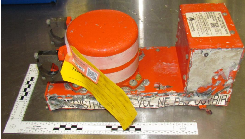
Figure A2: Recovered CVR at the ATSB laboratories in Canberra, 16 November 2015
