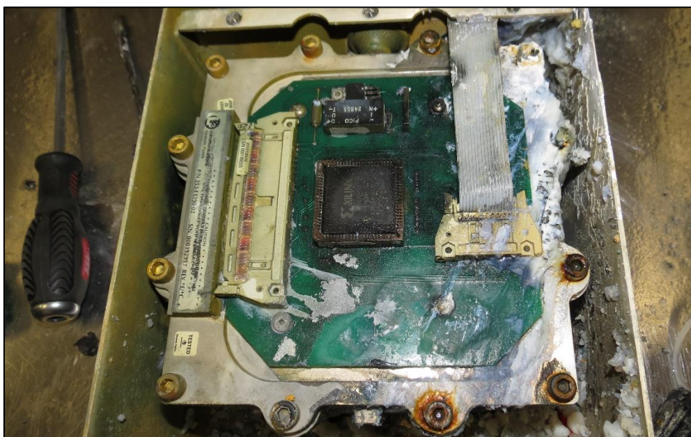
Figure B4: FDR memory module (16 November 2015)
