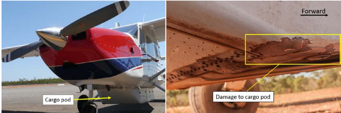
Figure 2: VH-MQI showing the cargo pod fitted to the aircraft (left) and damage sustained during the incident (right).
