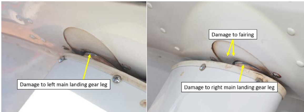
Figure 3: Damage to left main landing gear leg (left), and damage to the right main landing gear leg and fairing (right).
