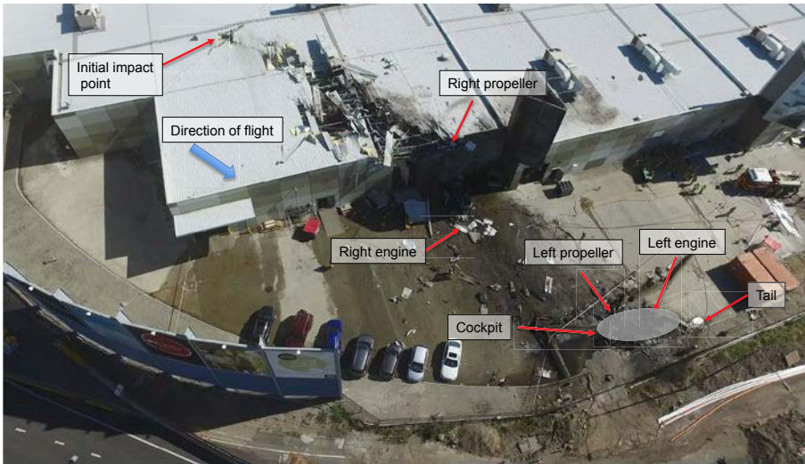
Figure 8: Accident site overview
