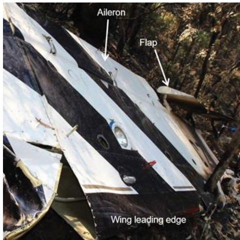
Figure 29: Left outboard wing, looking from the wingtip inboard and showing the lower surface of the wing from in-flight break-up involving PZL Mielec M18A Dromader aircraft (AO-2013-187)
