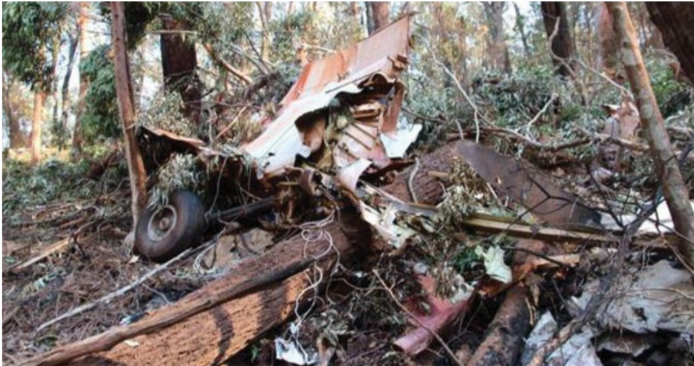
Figure 28: Main wreckage from in-flight break-up involving PZL Mielec M18A Dromader aircraft (AO-2013-187)
