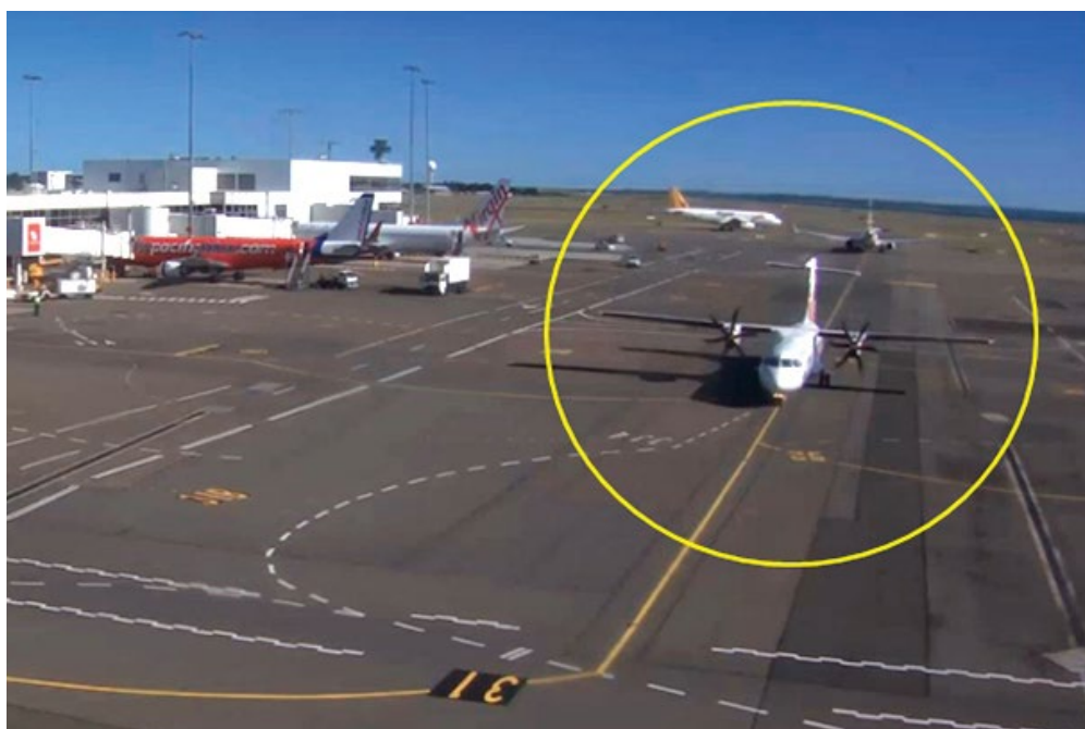
Figure 9: CCTV image showing VH-FVR (circled) taxiing inbound at Sydney Airport on 20 February 2014 following the in-flight pitch disconnect. Note the angle of the horizontal stabiliser relative to the wings.
