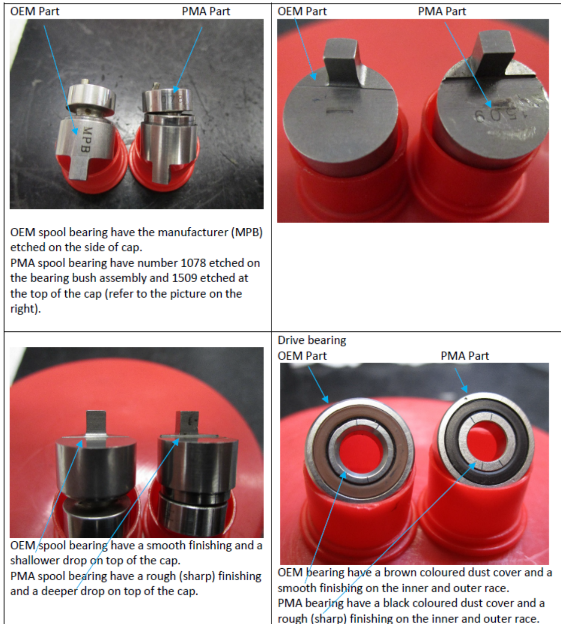
Figure 4: Comparison of OEM and PMA bearings
