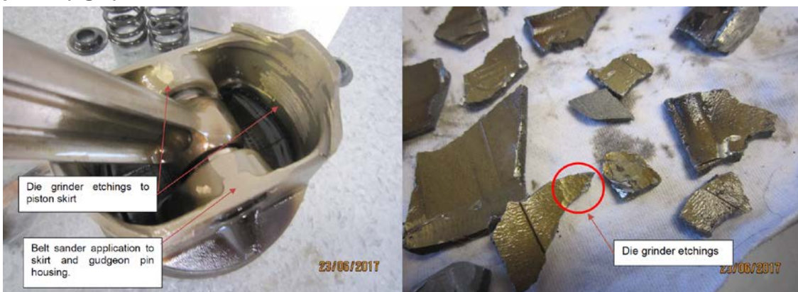
Figure 3: Belt sanding and die grinding of a piston (left) and fragments of the number five piston (right).
