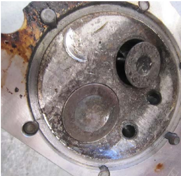
Figure 4: Cylinder five combustion chamber face showing damage and the bent exhaust valve.
