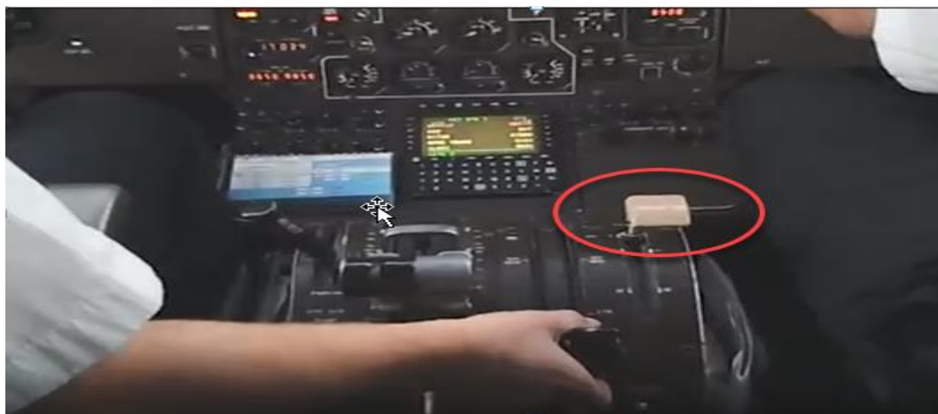
Figure 1: Location of flap lever on ATR72
