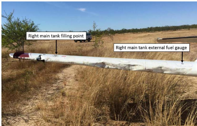
Figure 2: Damage to right wing
