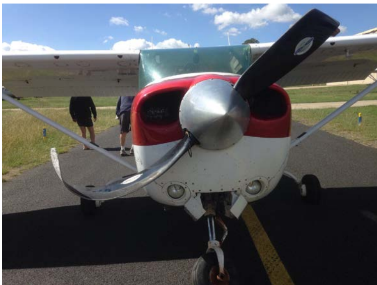
Figure 7: VH-JXX showing damage to the propeller and nose landing gear
