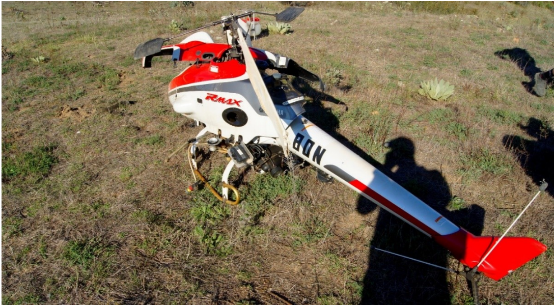
Figure 2: Damage to the RMAX
