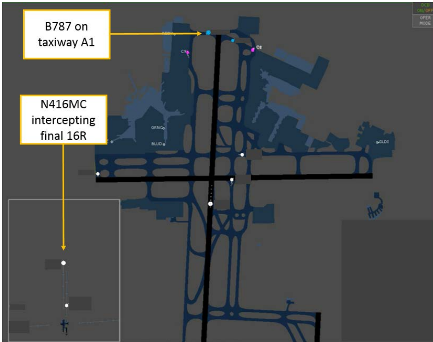
Figure 3: Infringement of the 16R glideslope critical area
