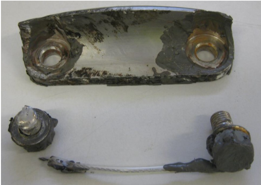
Figure 1: Anti-flap stop and securing hardware.
