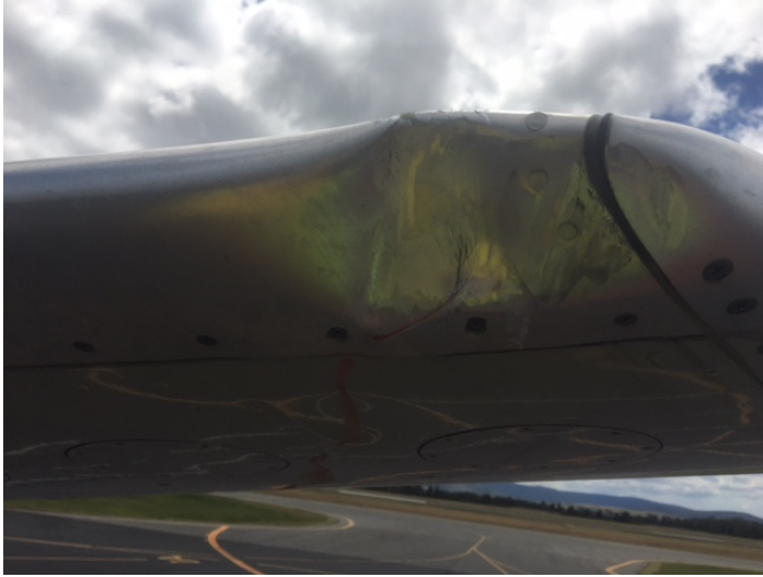
Figure 9: Damage to VUP left horizontal stabiliser
