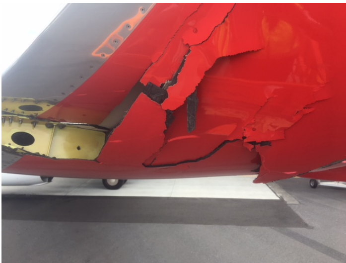
Figure 8: Damage to YFT left winglet
