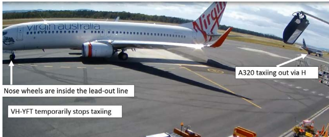
Figure 4: YFT stopped taxiing during the turn out of bay 3
