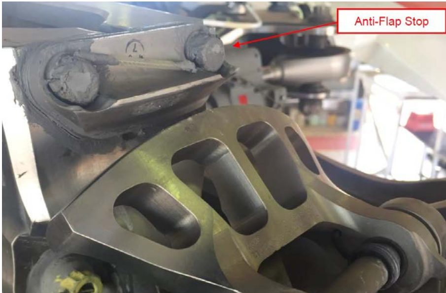
Figure 2: Anti-flap stop secured to the main rotor hub.
