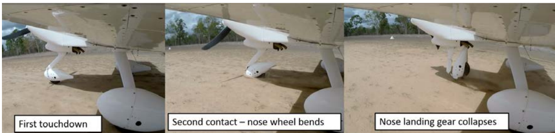
Figure 2: Landing sequence with collapse of nose landing gear
