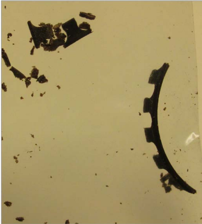
Figure 2: Pieces of the failed phenolic bearing cage
