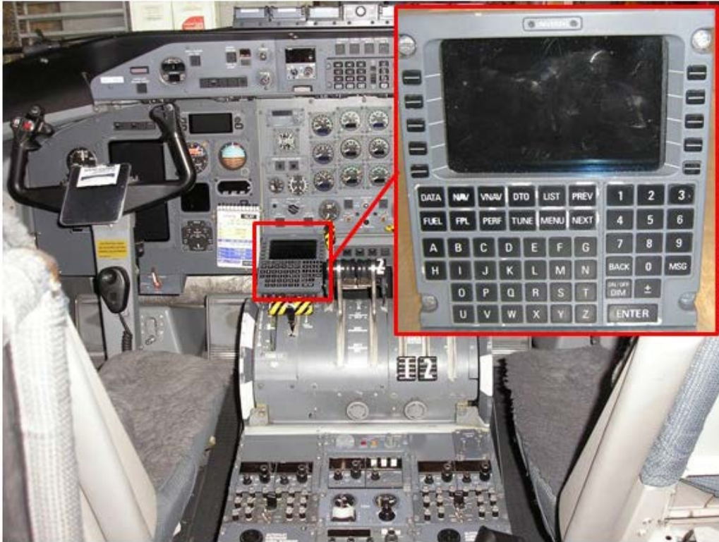
Figure 1: DHC-8-315 instrument panel showing the location of the FMS on the captain's side of the centre console (detailed view of the FMS at inset)
