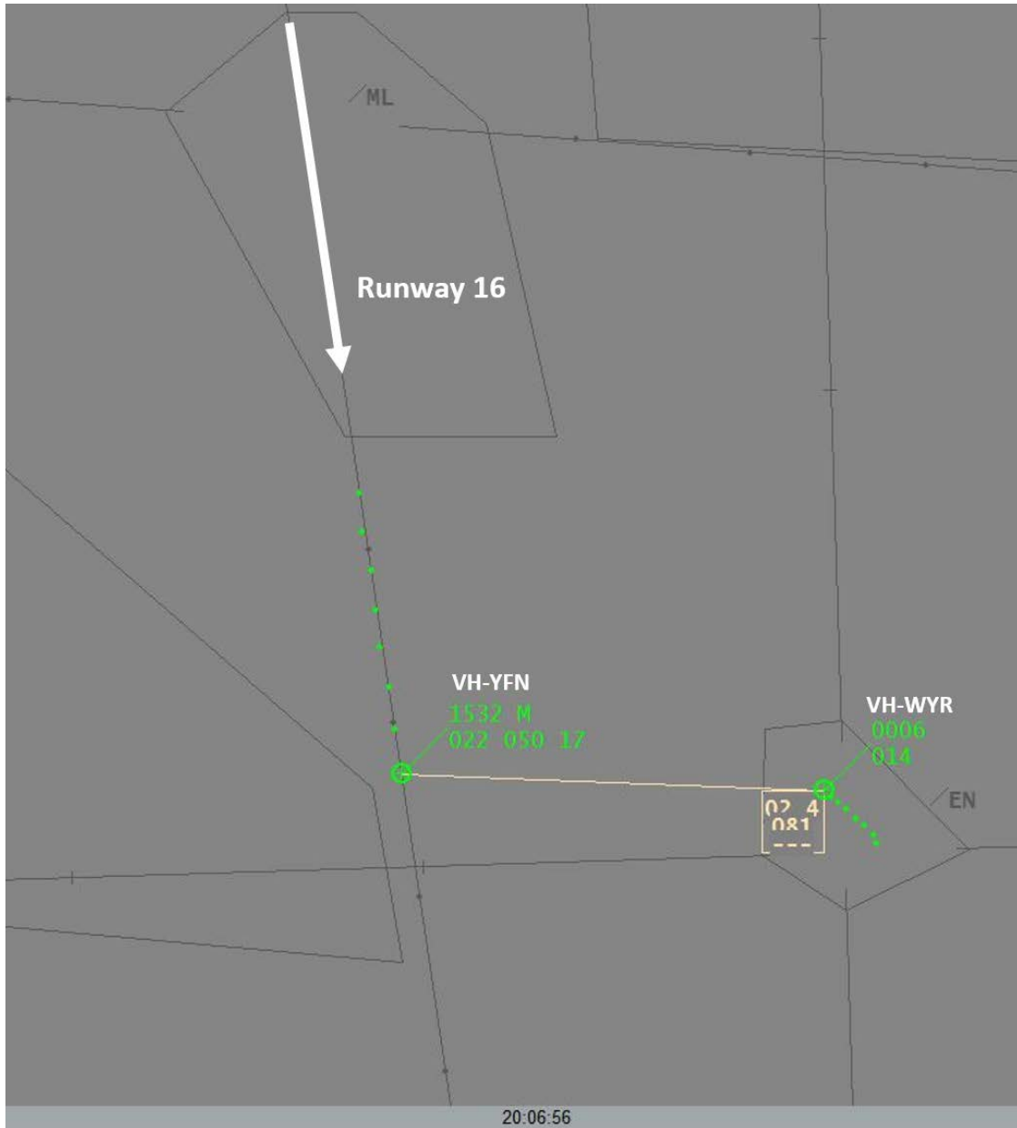
Figure 3: Air traffic control surveillance image at 0706:56, showing VH-YFN 2.4 NM (4.4 km) from and 800 ft above VH-WYR at Essendon Airport 12
