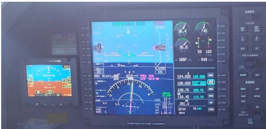
Figure 7: Electronic standby indicator and main PFD in flight (not OWA)
