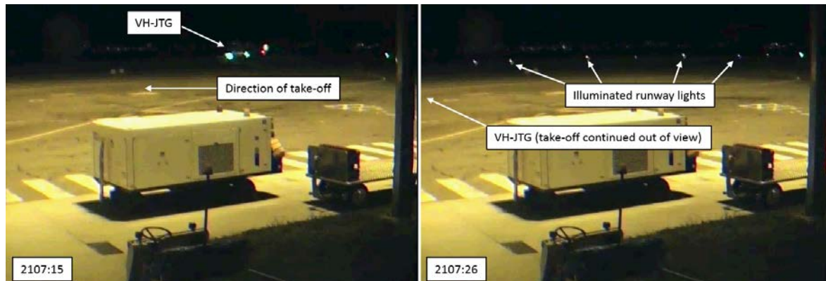
Figure 2: Take-off run of JTG on 19 August showing runway lights not activated (left) and then activated (right)
