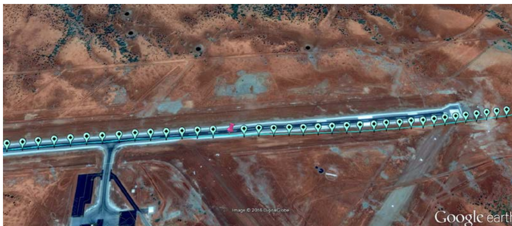
Figure 2: Deviation of OWA (travelling from left to right) from runway centreline showing the estimated point of the radalt failure (in pink)
