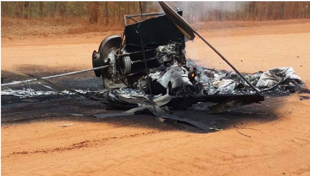
Figure 4: Accident site showing VH-PFX destroyed by post-impact fire
