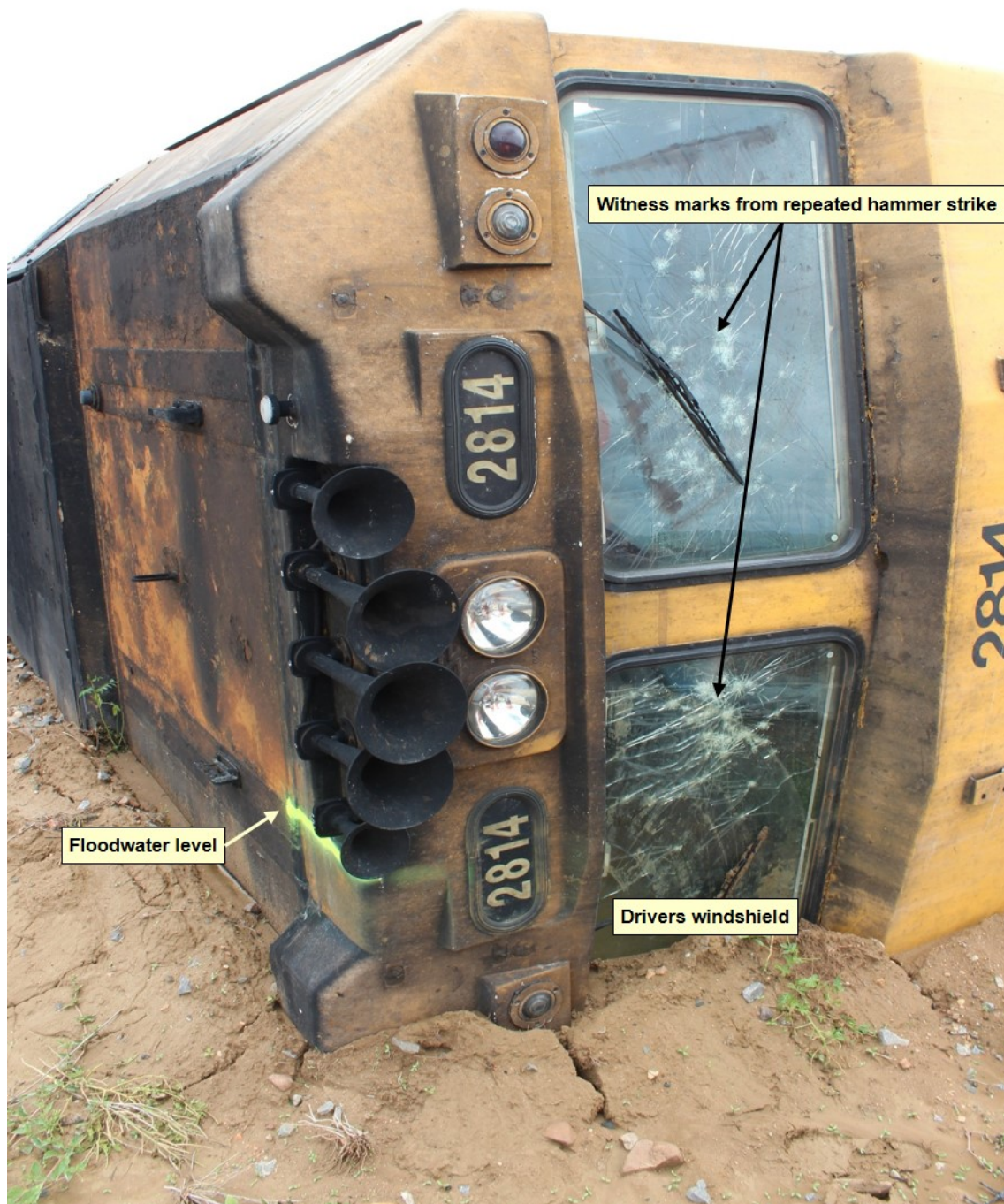
Image of leading locomotive 2814 in its final resting place and indicative water level. The image displays repeated attempt by train crew to smash out the windscreens with the emergency hammer. Source: Queensland Rail
