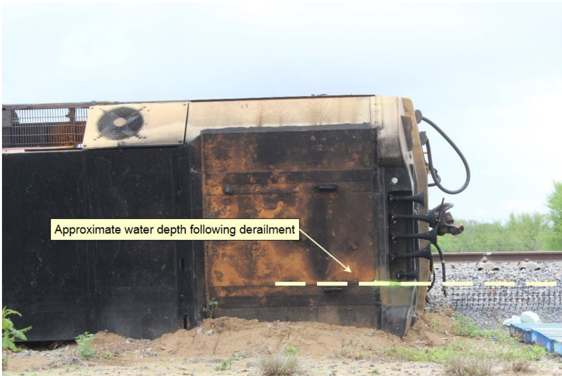
Watermark on the locomotive indicating the depth of the floodwater. Source: Queensland Rail
