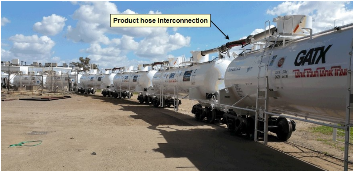
Image of a GATX tanker wagons coupled in a string and the product hoses interconnecting each vessel. Source: Incitec Pivot
