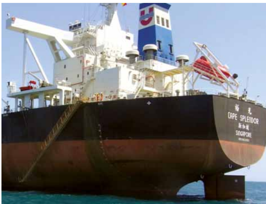
Figure 10: Cape Splendor's accommodation ladder
