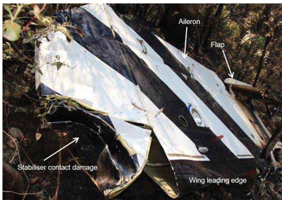
Figure 7: Outer section of left wing of VH-TZJ
