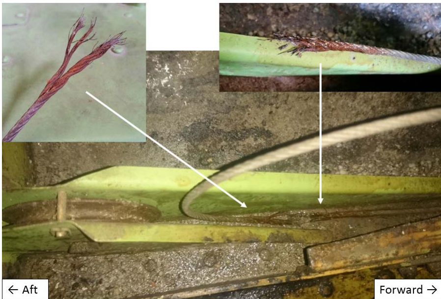
Figure 4: VH-TTD broken flap cable
