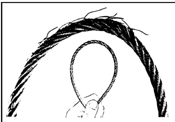
Figure 5: Cable inspection technique
