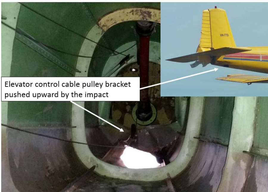
Figure 2: VH-TTD elevator control cable pulley
