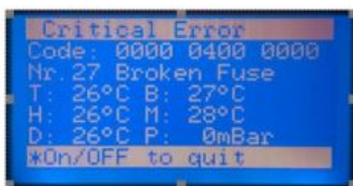
Figure 2: Error message from oven on N35953
