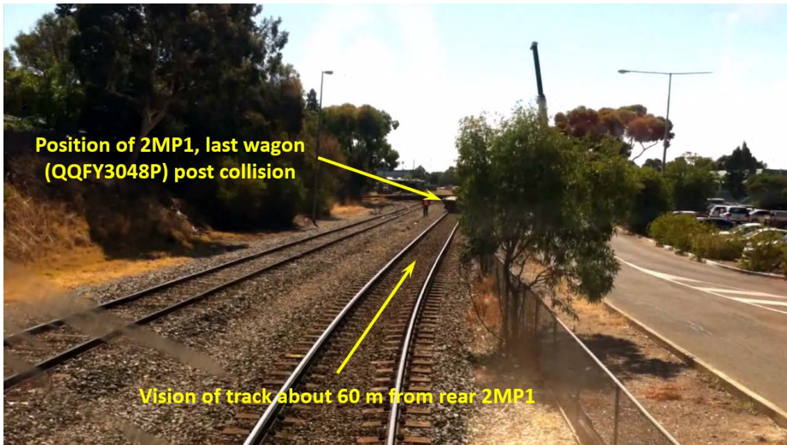
Figure 6: Cab view post image reconstruction, about 60 m from rear end of 2MP1
