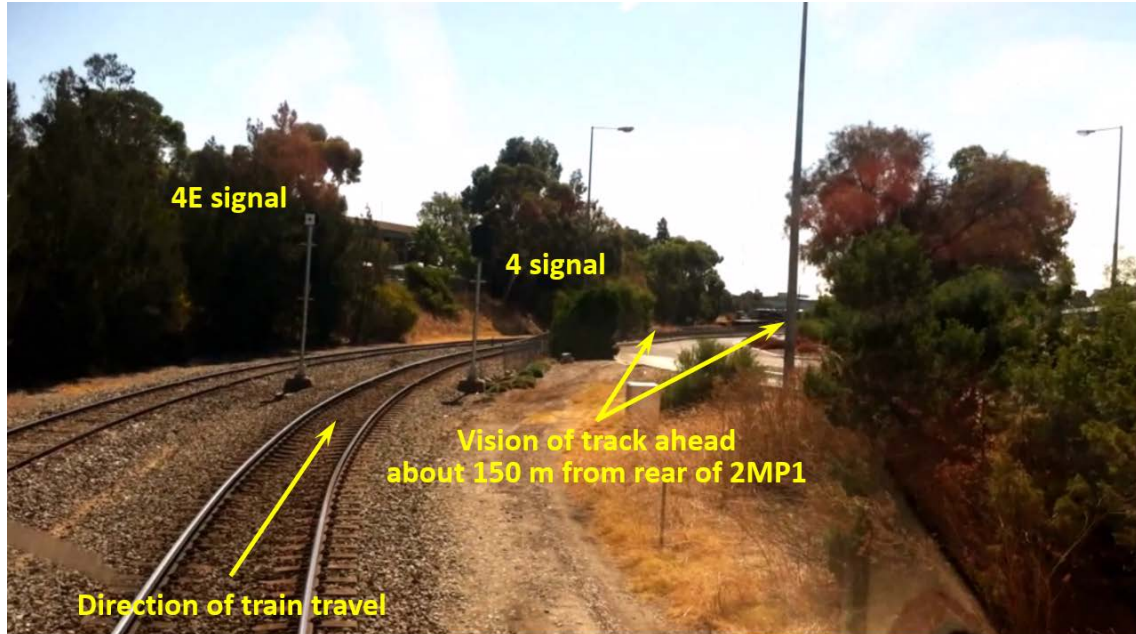
Figure 4: Cab view post-collision reconstruction, about 150 m from the rear end of 2MP1
