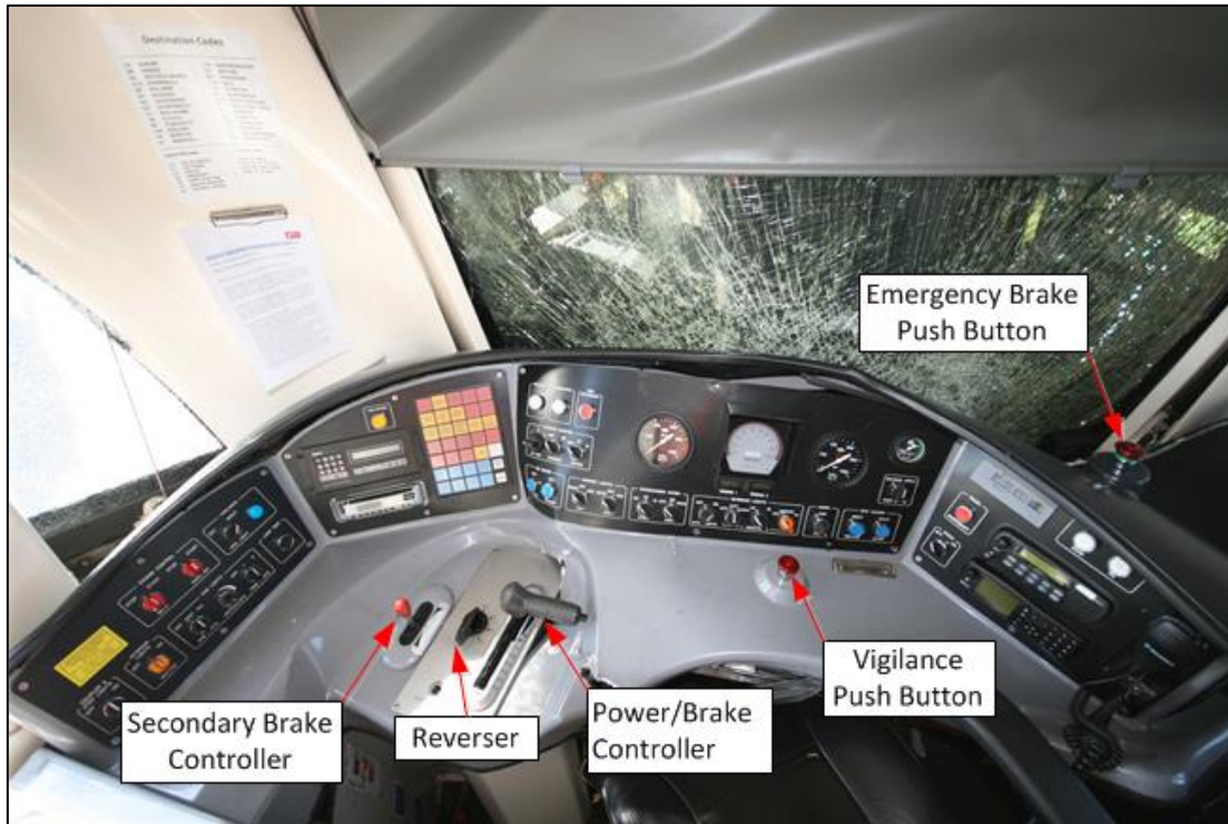
Figure 10 - Driver control console showing the main controls
