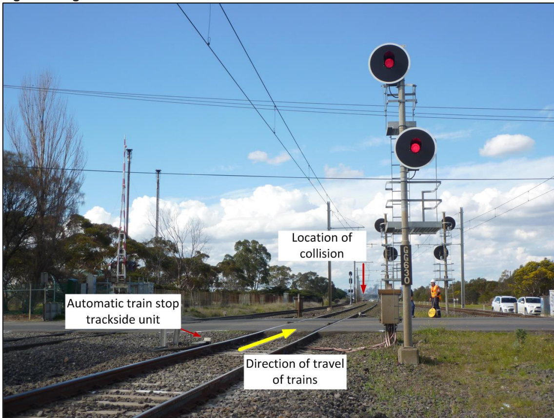
Figure 3: Signal GG630 and indication of collision site
