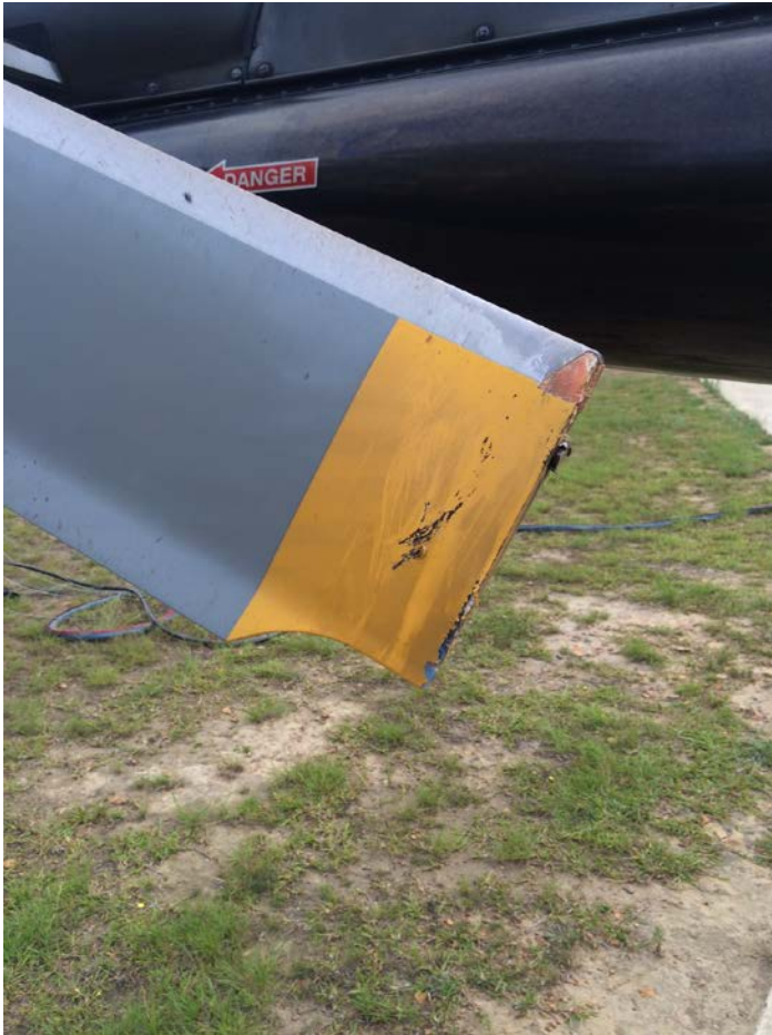
Figure 2: Damage to VH-NPS tail rotor
