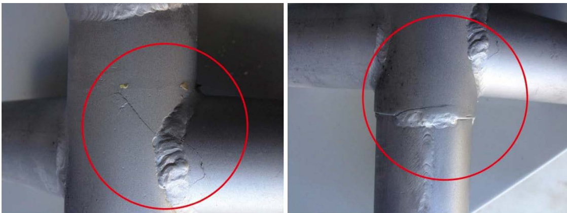
Figure 4: Cracks in the welded tube junction of the stabiliser mount
