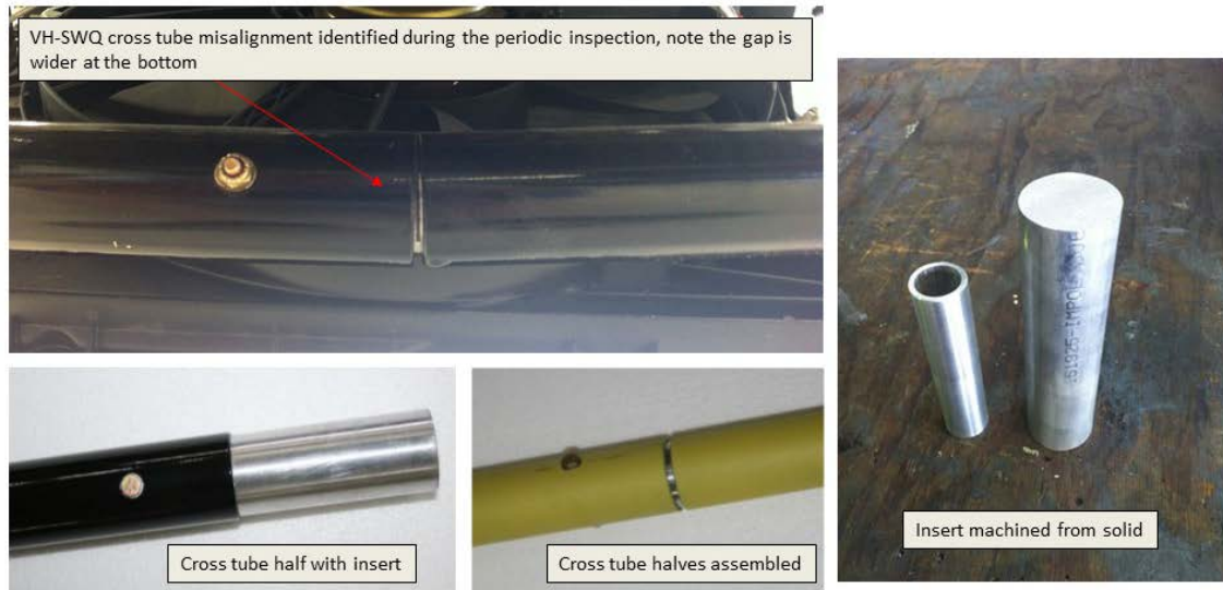
Figure 5: VH-SWQ cross-tube and inserts
