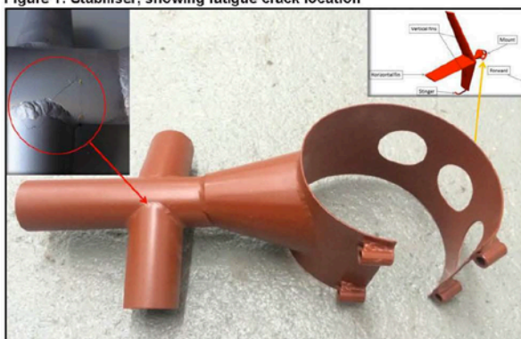
Figure 1: Stabiliser, showing fatigue crack location
