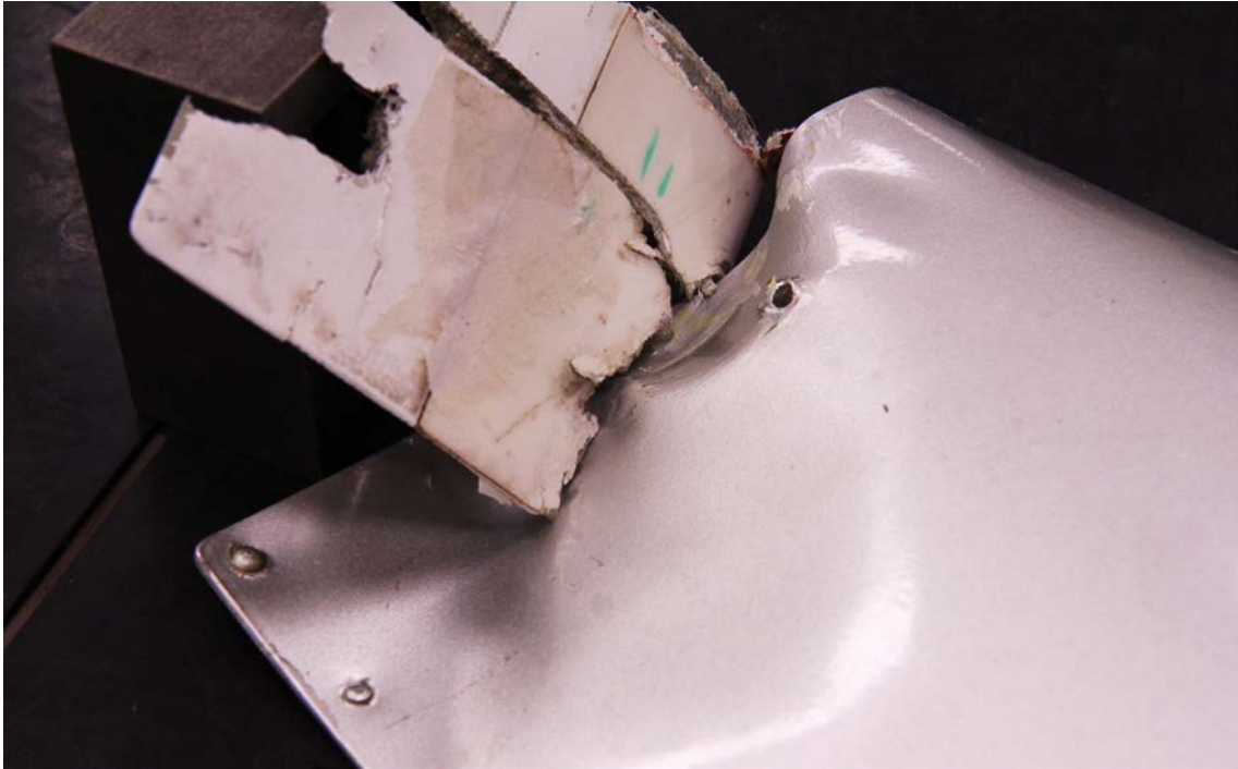
Figure A2: Matching witness marks indicate that a tail rotor blade contacted the lower fin
