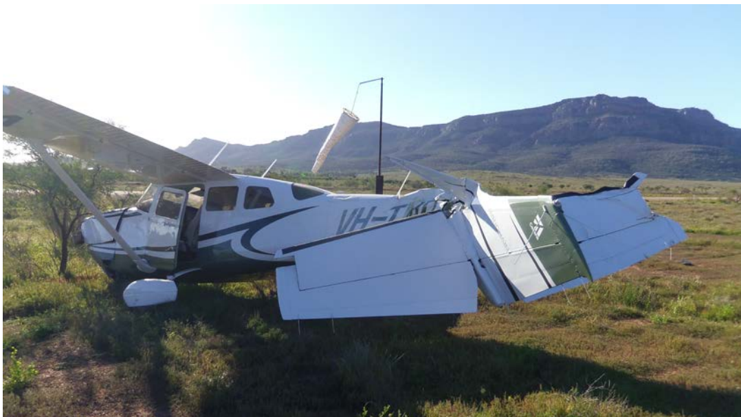
Collision with terrain involving a Cessna C206 at Rawnsley Park, SA on 2 August 2014 (ATSB investigation AO-2014-135) – rear fuselage and tail damage. Source: South Australian Police.
