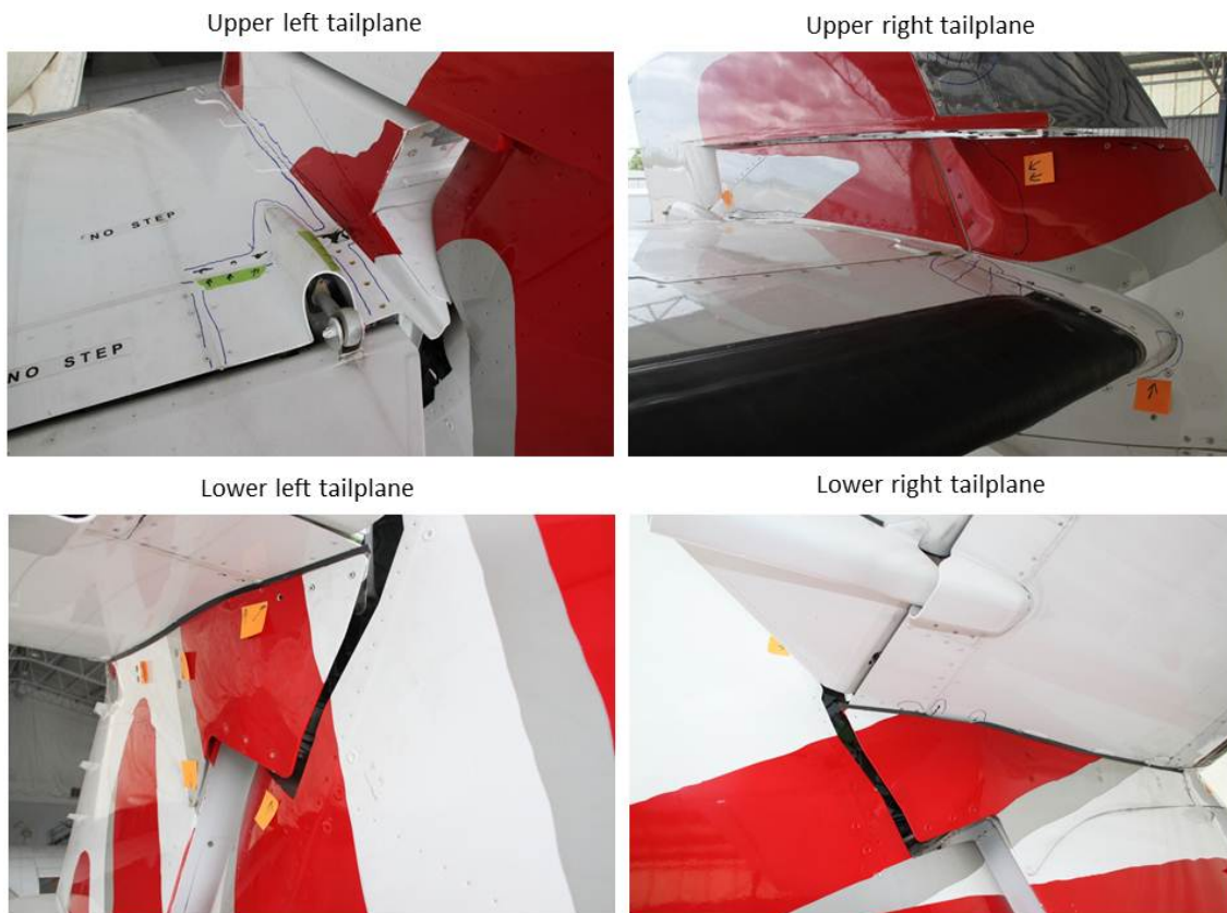
Flight control event involving an ATR72, 47 km WSW Sydney Airport, NSW on 20 February 2014 (ATSB investigation AO-2014032) - tailplane external damage (indicated by marks and stickers). Source ATSB.
