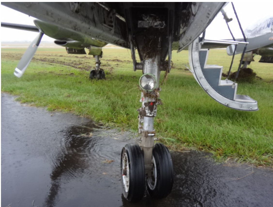
Runway excursion involving a Fairchild SA226 at Archerfield Airport, Qld on 23 January 2014 (ATSB investigation AO-2014-016) – skid marks in the grass following a runway veer off in wet conditions.
