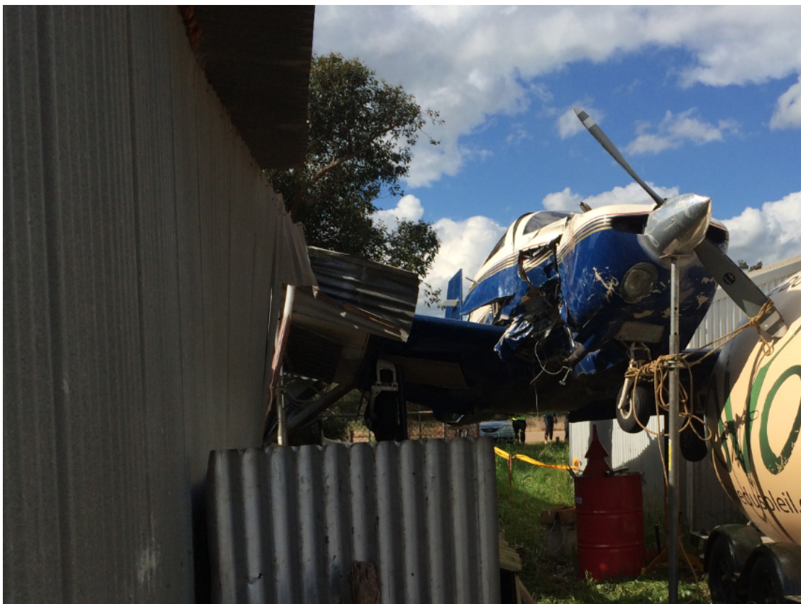
Collision with terrain involving a Mooney M20J, at Northam (ALA), Western Australia on 5 September 2014 (ATSB investigation AO-2014-148). - accident site and damage to the aircraft. Source: Operator.
