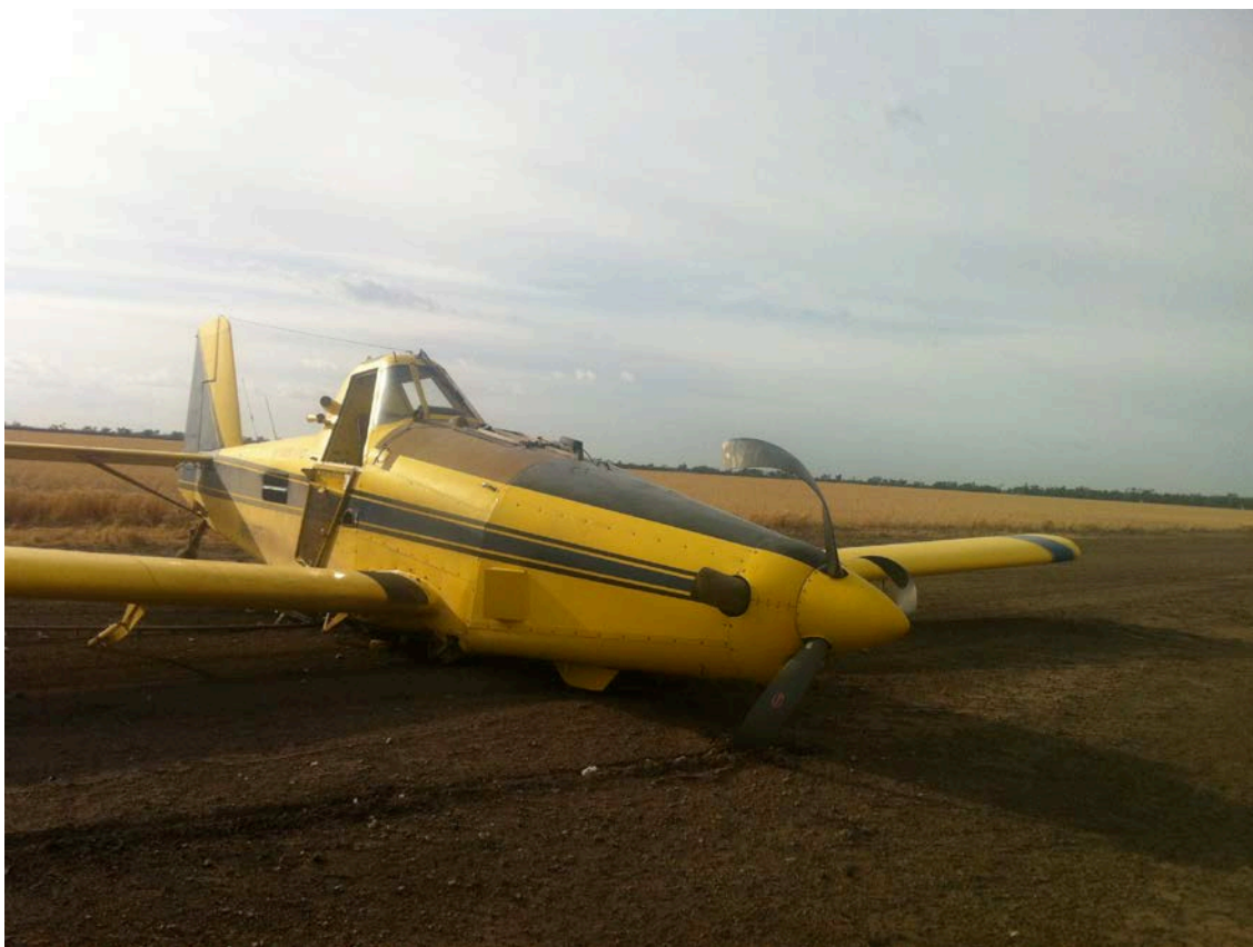
Collision with terrain involving an Air Tractor AT-502B, 45 km west of Moree Airport, NSW on 18 December 2014 (ATSB investigation AO-2014-191) - Damage to aircraft. Source: Pilot.
