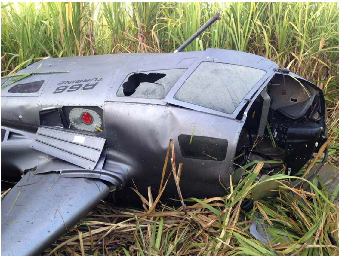
Wirestrike involving Robinson R66, near Giru, Qld. on 20 August 2014 (ATSB investigation AO-2014-142) – aircraft damage. Source: Operator.
