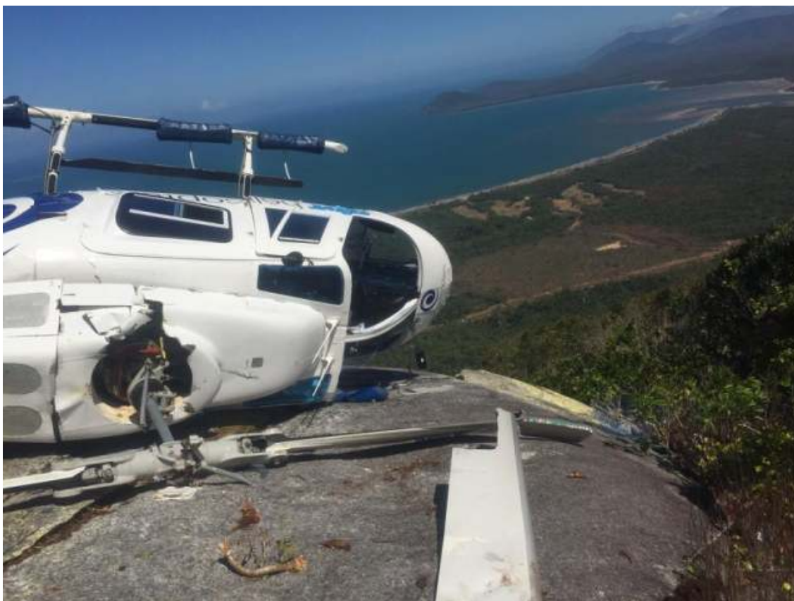
Loss of control during landing, involving a Bell 206B3 9km south-east of Cooktown Airport (Mount Cook), Queensland, 7 October 2014 (ATSB investigation AO-2014-161) – dynamic rollover accident on Mount Cook. Source: Queensland Police.
