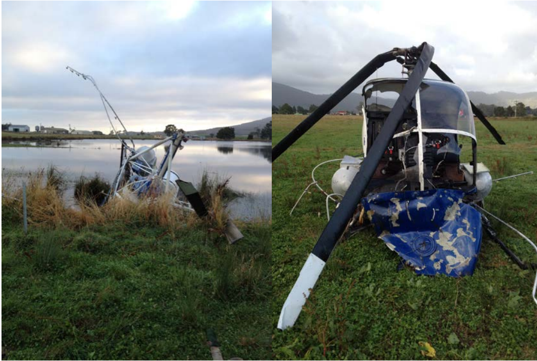
Collision with terrain involving a Hughes 269C, 55 km NE Launceston Airport, Tasmania on 23 February 2014 (ATSB investigation AO-2014-030) – damage of the aircraft. Source: Operator.
