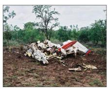
The wreckage was located about 4 km east of the aerodrome. An examination of the wreckage indicated that the aircraft impacted the ground inverted in a steep nose-down attitude. The accident was not survivable. The wreckage was consistent with a loss of control situation, but the likely reason for the loss of control could not be determined.
