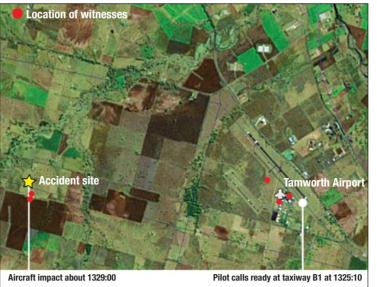
and increasing airspeed. The aircraft flight path reported by witnesses was found to be consistent with the effect of abnormal rudder and/or aileron trim tab settings.
