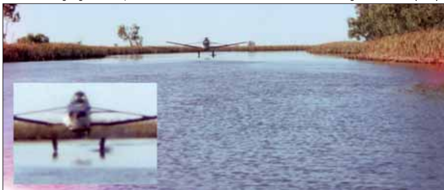
Cessna 188B Agwagon aircraft, VH-ZIP at water-ski area. Note left main wheel contacting water surface (inset)
