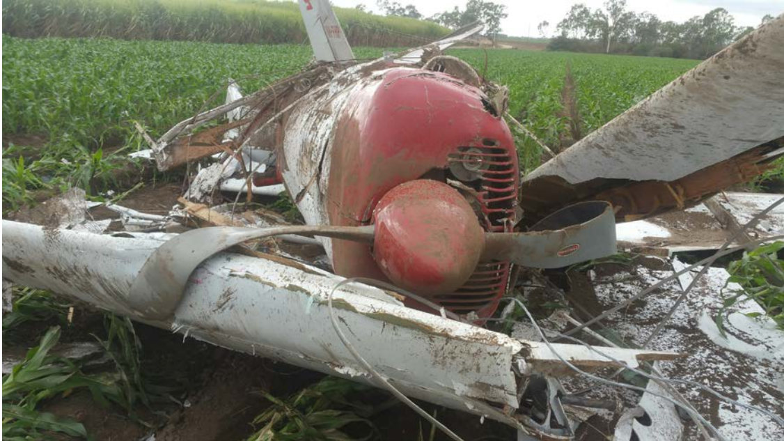
Figure 2: Photo of VH-FHP at the accident site showing damage to the aircraft and wires
