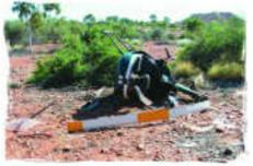
During the flight some cattle were observed outside the fenced area and the pilot descended to direct the cattle back towards the fence. The passenger reported that the pilot had just commenced to climb higher, at his request, when the helicopter collided with a single-wire powerline. The wire was not severed and the helicopter pitched nose down and the main rotor severed the tail boom. The helicopter collided with the ground. There was no fire.
