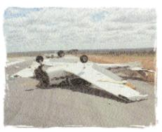
The nose of ZIR pitched steeply upwards and the aircraft became inverted, striking the runway in a nose low attitude while the nose of ZIB pitched downwards with the aircraft landing heavily on its nose wheel. Both aircraft came to rest on the runway.
