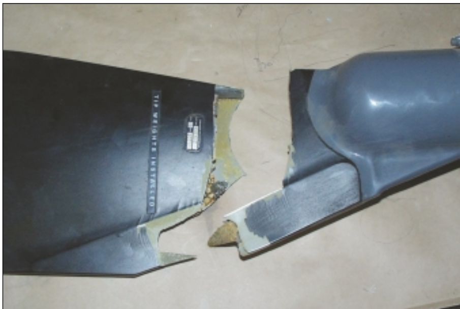
Figure 1: The broken rotor blade
