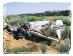
It was determined that the aircraft entered a spin. The rotation of the spin was subsequently arrested, however the aircraft impacted the ground as it was accelerating during the pull out from a dive at the end of spin recovery. The landing gear and flaps were extended at the time of the accident.
