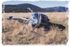
The investigation determined that the drive spline and coupling from the main gearbox to the hydraulic pump had failed due to lack of lubrication. This resulted in the loss of hydraulic power to the controls and the loss of main rotor RPM indication.
