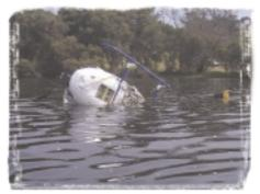
a bank to right the helicopter unexpectedly lost height which the investigation concluded was consistent with it entering an area of strong turbulence.
