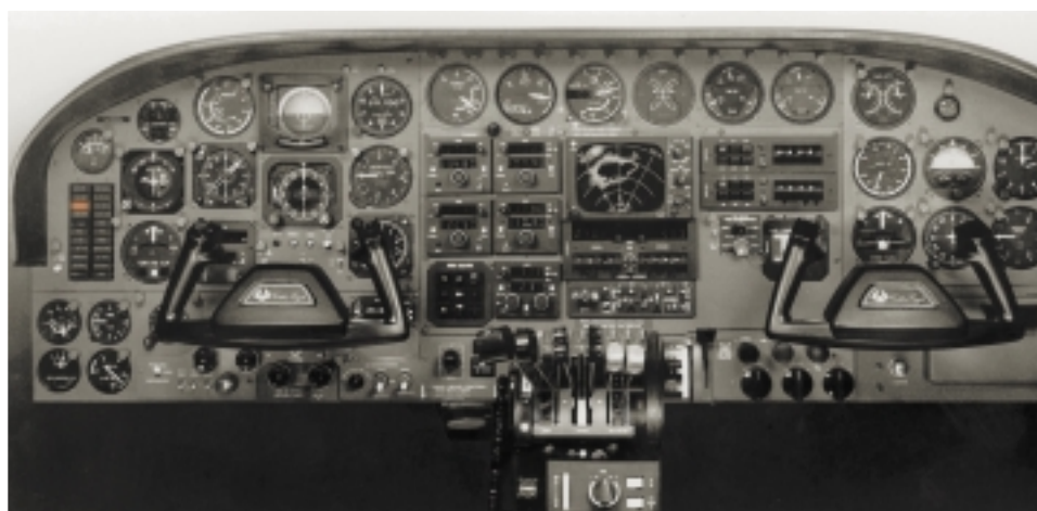
Instrument panel of a Cessna 421 Golden Eagle showing the position of the cabin altitude warning light (shown in red). Below it are the cabin altitude and cabin differential indicator and the cabin VSI gauges.
