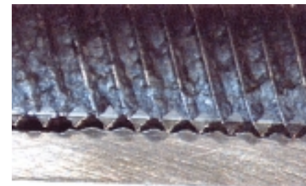
A cross section view of the Cessna 402 trim tab actuator.
