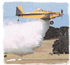
The aircraft approached the drop site ten knots faster than recommended, and during the water release, the nose pitched up and the aircraft entered a climb. The nose continued to pitch up with an increasing climb angle. There was no evidence that the pilot had made any elevator input to reduce the steepness of the climb.
