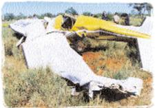
The pilot was positioning the aircraft to cut off a mob of sheep that had broken away from the group when the aircraft impacted the ground in a near vertical attitude at low forward speed. No evidence of any mechanical defect was found.
