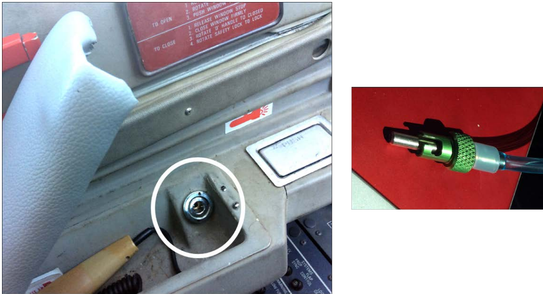
Figure 1: Oxygen port beneath pilot's armrest and associated oxygen fitting
