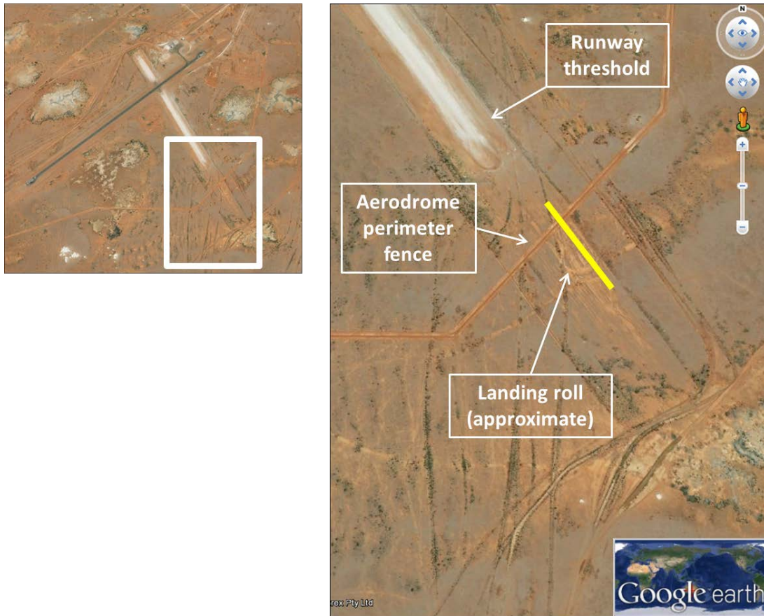
Figure 3: Coober Pedy Aerodrome with approximate position of the aircraft ground roll relative to the aerodrome perimeter fence and runway threshold
