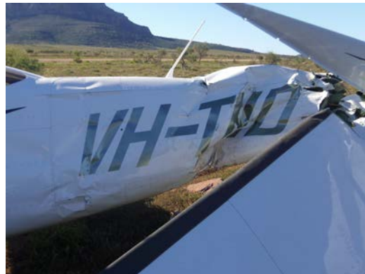
Figure 4: Rear fuselage and tail damage
