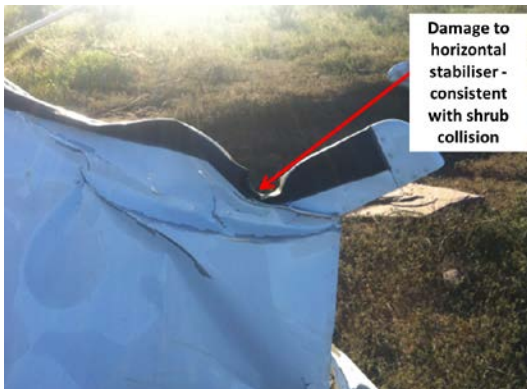
Figure 3: Damage to horizontal stabiliser
