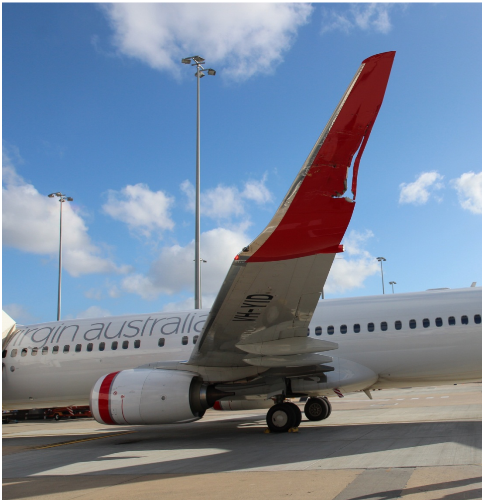
Collision during pushback operations between Boeing 737-800 (VH-YID) and Airbus A320-200 (VH-VGR), Melbourne Airport, Victoria (ATSB investigation AO-2013-033)
