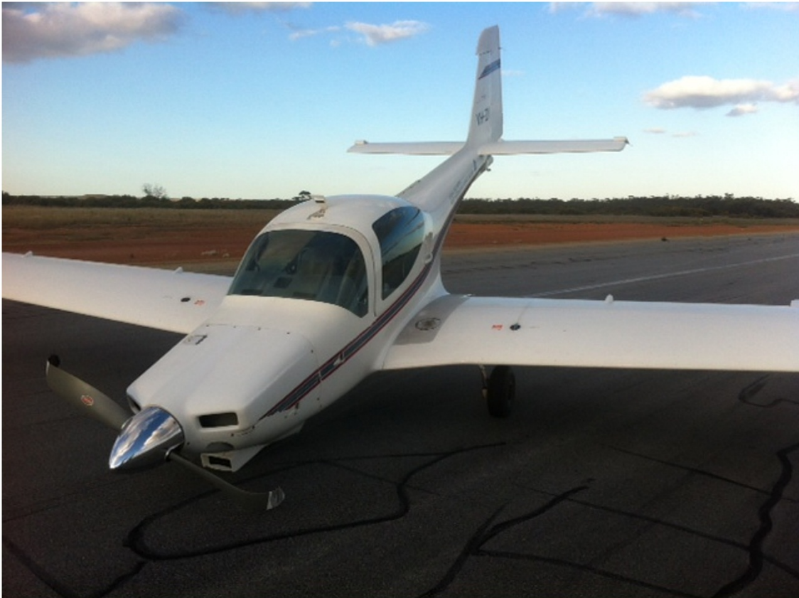
Hard landing involving a Grob G-115 (VH-ZIV), at Merredin, Western Australia (ATSB investigation AO-2013-178)
