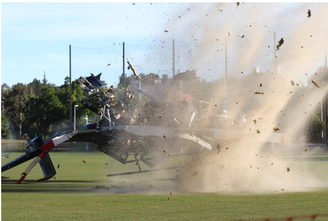
Collision with terrain involving a Bell 206L helicopter (VH-VDZ), Melbourne, Victoria (ATSB investigation AO-2013-199) – picture shows right roll and main rotor ground strike
