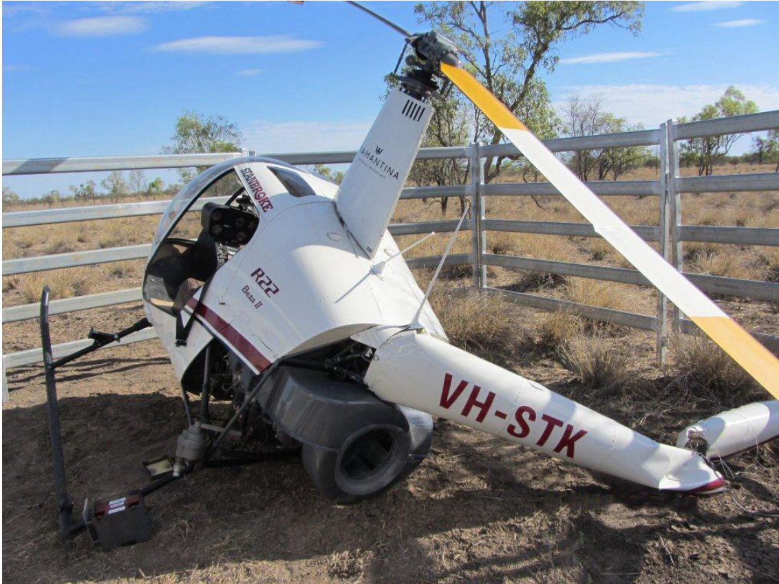
Total power loss involving a Robinson R22 helicopter (VH-STK), 155 km south-west of Normanton, Queensland (ATSB investigation AO-2013-211)
