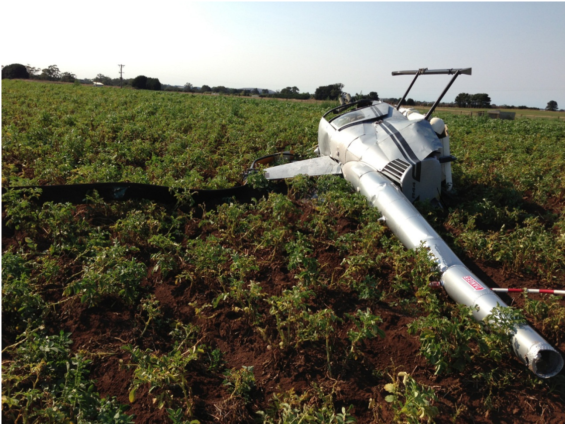
Wirestrike involving a Robinson R44 helicopter (VH-HGF), near Ballarat, Victoria (ATSB investigation AO-2013-042)
