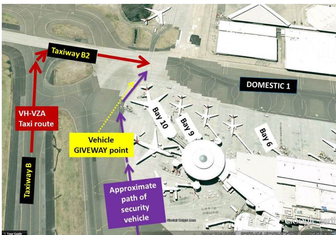
Ground proximity event between Boeing 737-800 (VH-VZA) and a security vehicle at Sydney Airport, New South Wales (ATSB investigation AO-2013-135) – diagram shows the relative positions of the aircraft and vehicle
