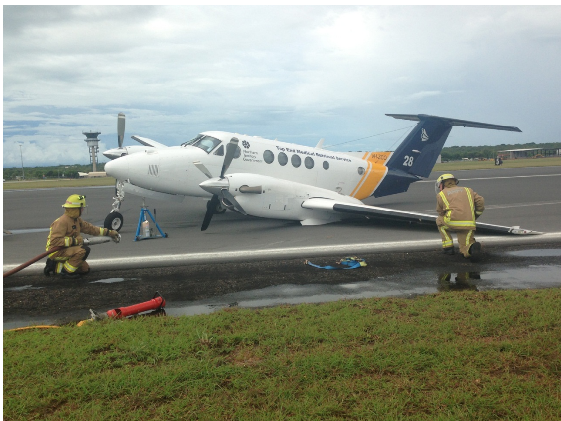
Left main landing gear collapse involving a Beech B200 King Air (VH-ZCO), at Darwin Airport, Northern Territory (ATSB investigation AO-2013-062)
