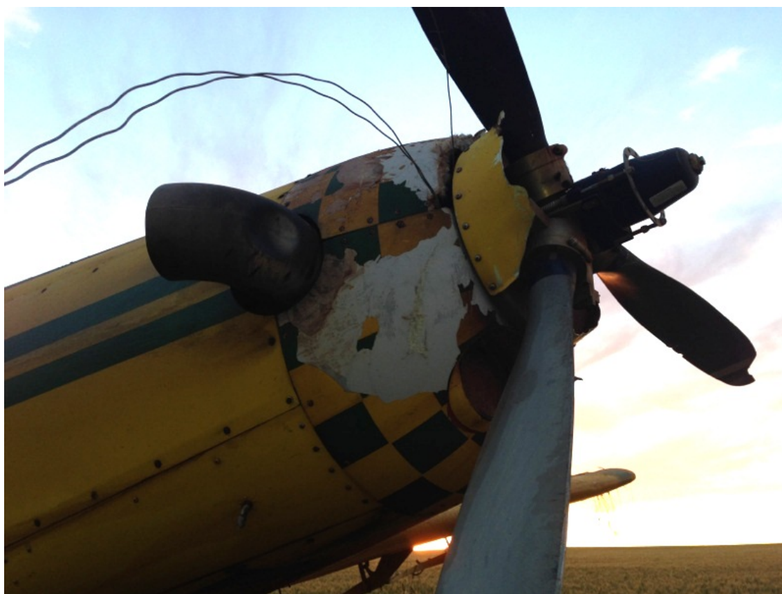
Wirestrike involving an Air Tractor AT-502 (VH-CJY), near Temora, New South Wales (ATSB investigation AO-2013-180)
