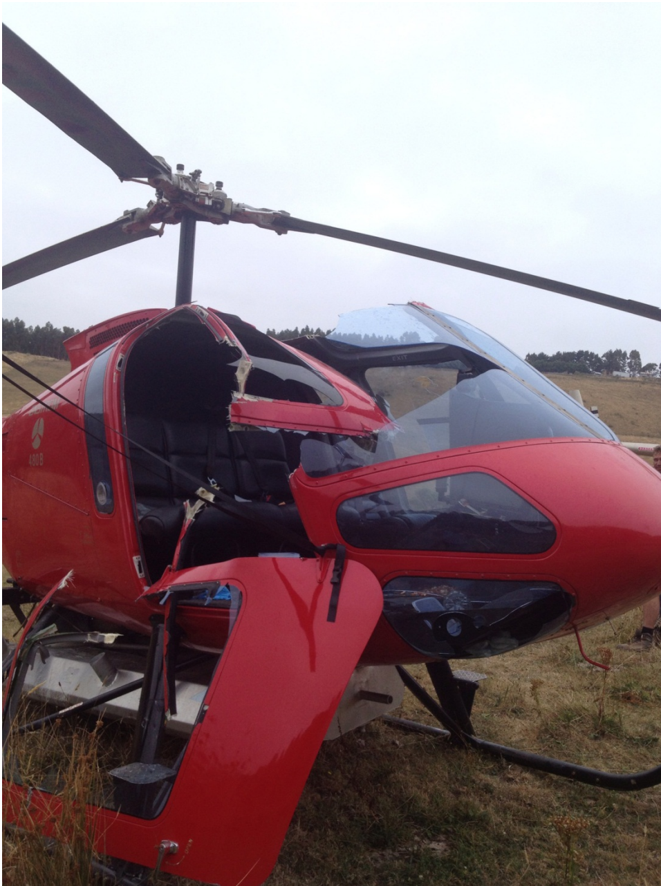
Wirestrike involving an Enstrom 480B helicopter (VH-VDC), near Ballarat, Victoria (ATSB investigation AO-2013-031)
