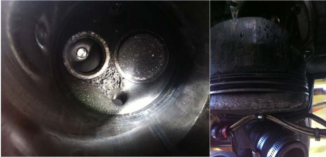
Figure 2: Damage to number three cylinder and piston
