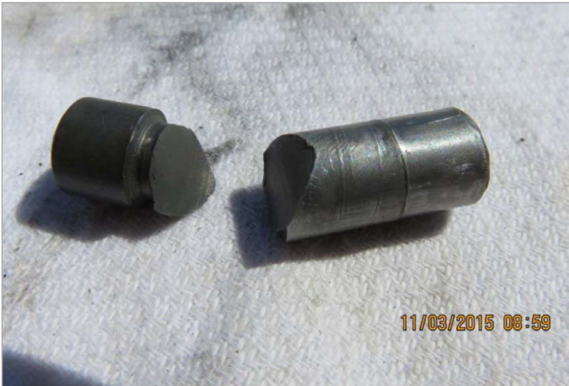
Figure 1: Failed nose landing gear downlock pin
