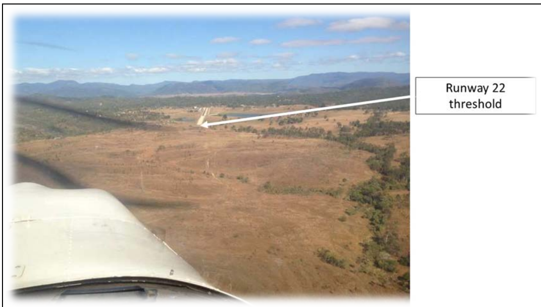
Figure 3: Approach to runway 22 at Lakeside Airpark. Note the unsealed and sealed portion of the runway. Also, note the difficulty in detecting the power lines on approach. Photo taken about a week prior to the accident
