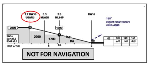
Figure 5a: Excerpt from the RNAV-U (RNP) runway 16 approach chart used by the operator showing vertical profile information
