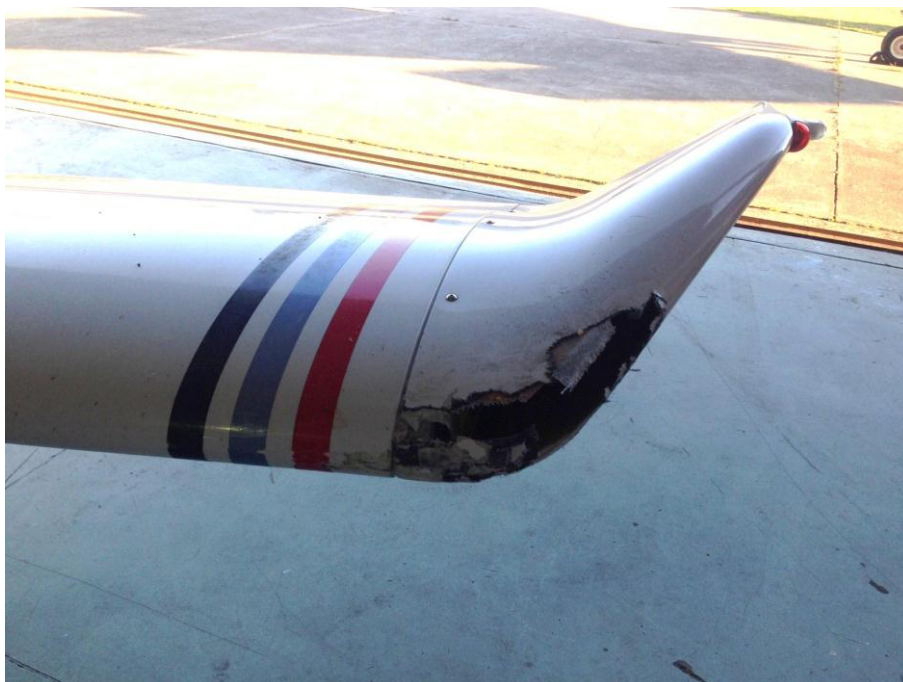
Figure 1: Left wingtip damage
