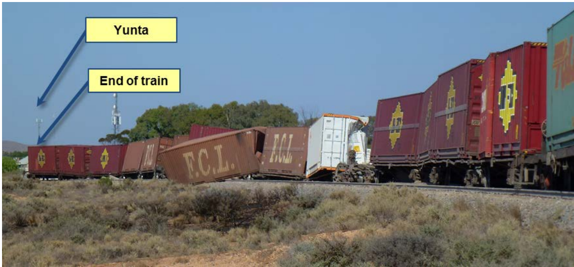
Figure 2: Derailed wagons at the end of train 3PS6
