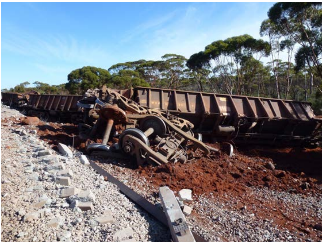
Figure 2: Train 4413 End of Train – Derailed Ore Wagons
