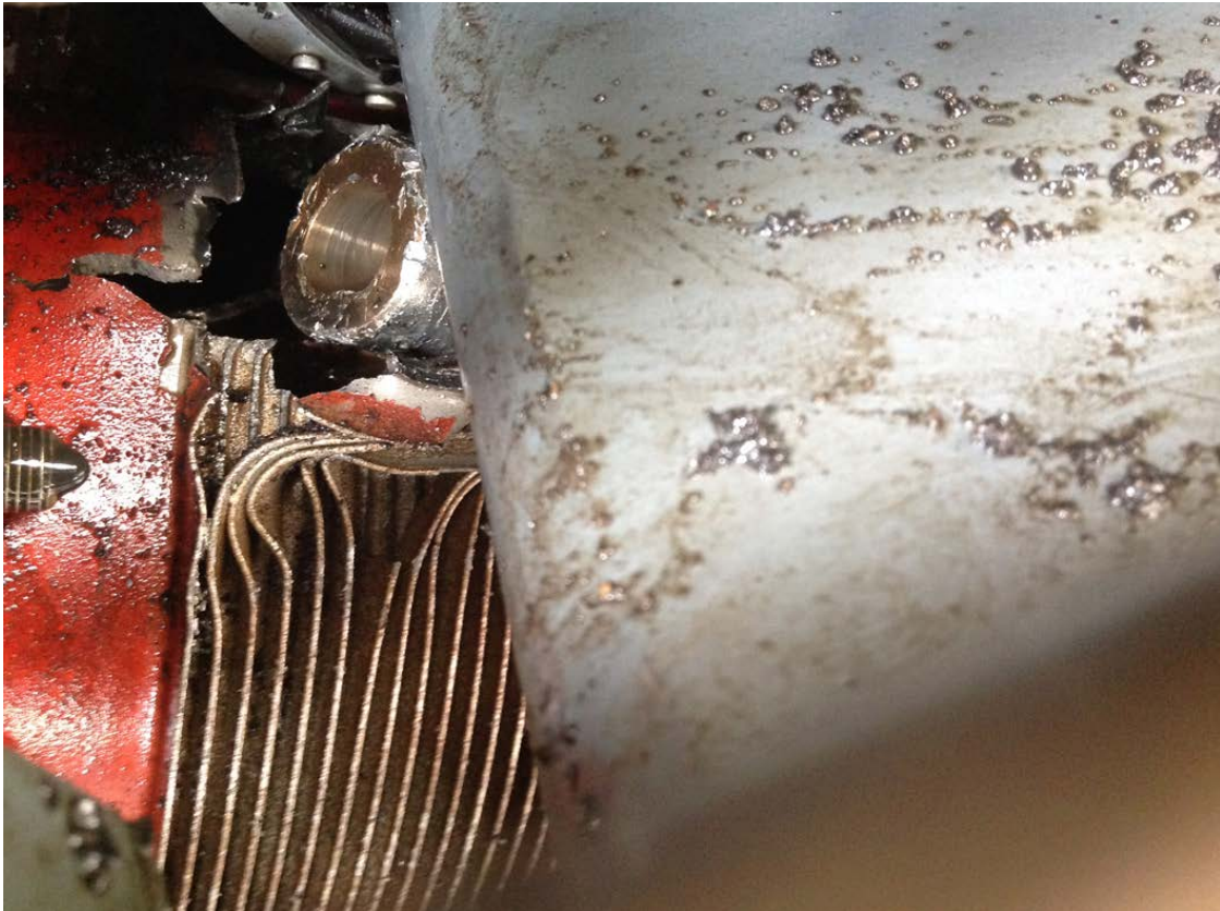
Figure 2: External view of damage to number five cylinder
