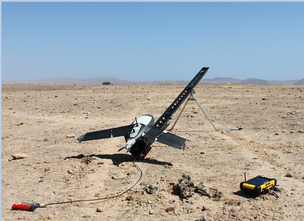
An example of the Gatewing RPA system on its launch rail. Source Wiki Commons
