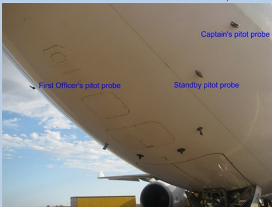
Locations of pitot probes. Source ATSB
