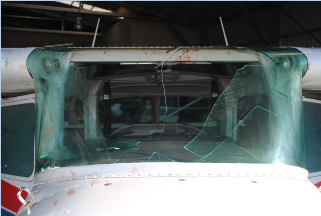
The result of an impact with a Flying fox, showing where the animal penetrated the windshield of the Cessna 152. Source: ATSB
