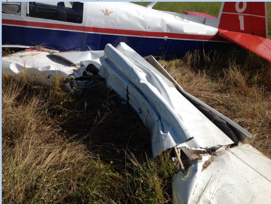
Damage to the Mooney M20J caused by striking a bull. Source: ATSB
