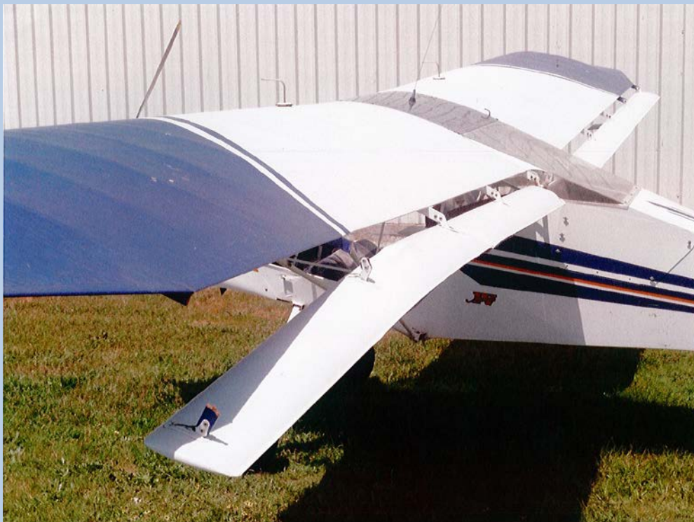
Damage caused by strike with an eagle. Source ATSB
