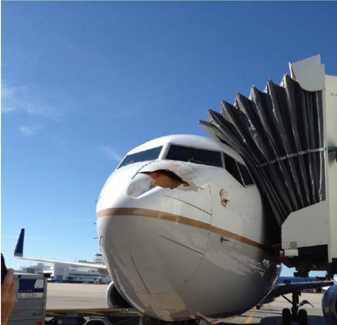
Damage to a Boeing 737-900 following a birdstrike on descent to Denver, US. Source: NTSB
